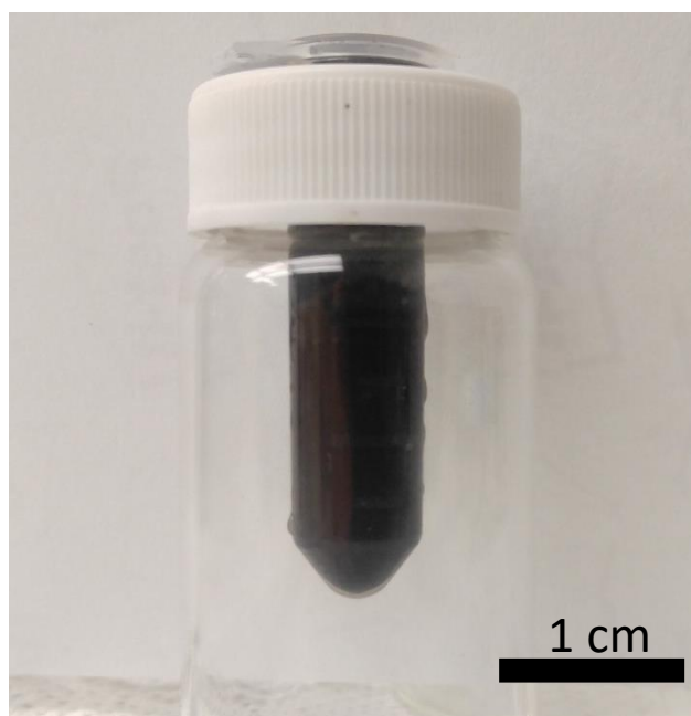
Figure 7.5: Digital image of the as-prepared N-MWrGO ink within a microcentrifuge tube
