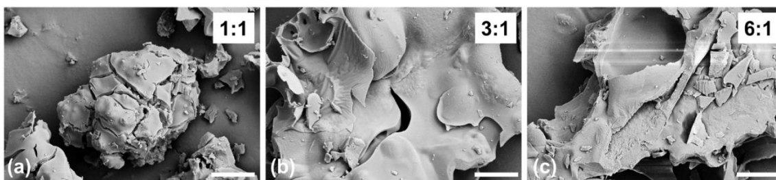
Supplementary Figure 3. Representative FE-SEM micrographs of BCNO compounds synthesized at 1000°C using a) 1:1, b) 3:1, and c) 6:1 of BA:M ratios. Scale bars in micrographs correspond to 10 \mu\text{m} .
