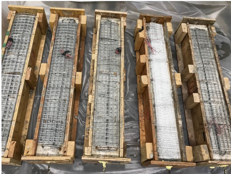
Figure 3. 13 Ferro Mesh Placed Before Casting of Mortar
