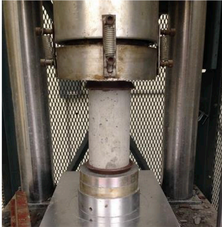
Figure 3. 8 Cylinder Placed Inside Compression Machine
