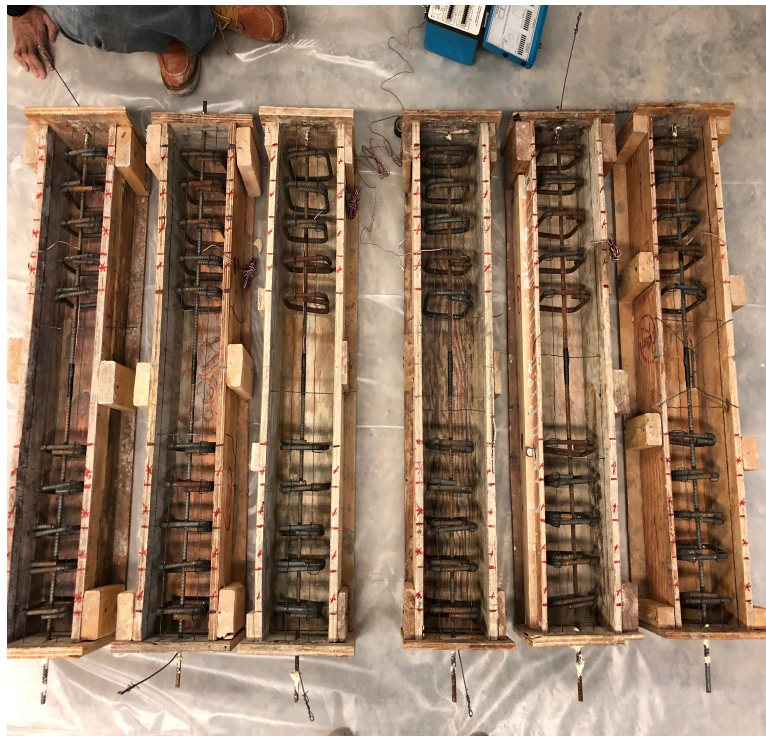
Figure 3. 10 Beam Molds with Shear Reinforcement Placed and Fixed
