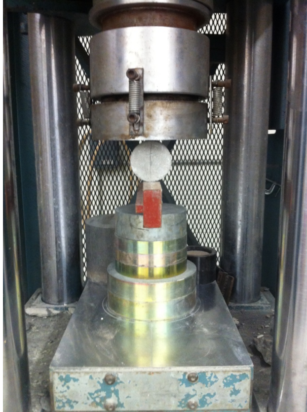
Figure 3. 6 Splitting Tensile Test
