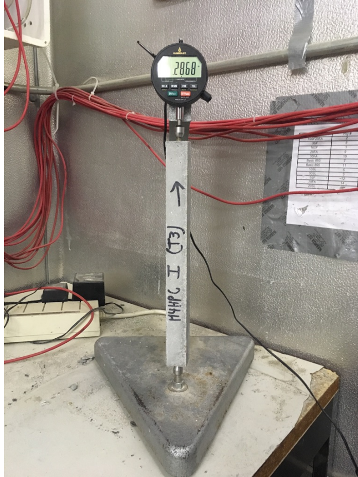
Figure 3. 7 Mortar Free Shrinkage Specimen Measurement
