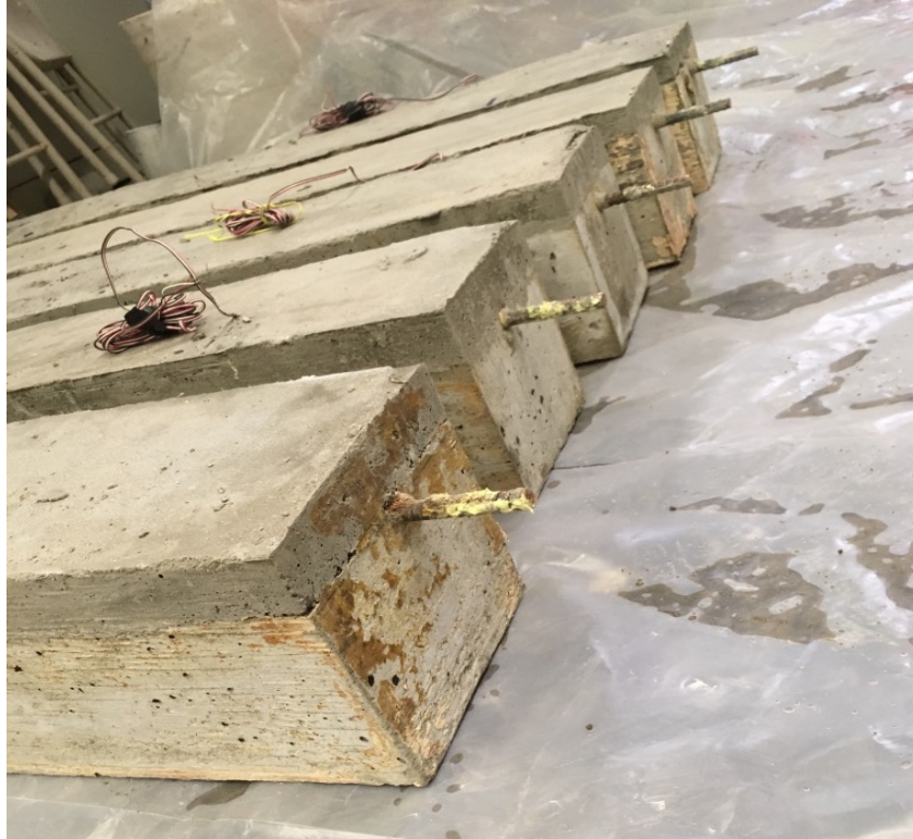
Figure 3. 14 Beams with Ferrocement Laminate
