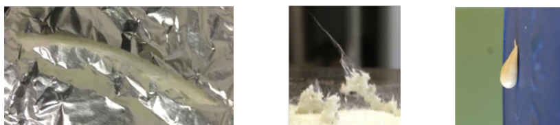
Figure 6.14 Synthesized inorganic polymers showing characteristics of conventional polymers: bending (left), fibril formation (middle), and flow (right).
