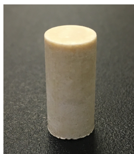
Figure 3.6 A picture of an inorganic polymer synthesized for monovalent system. The diameter is 10 mm and height is 20 mm.
