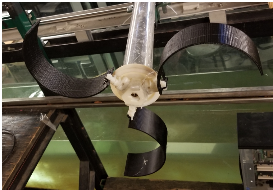
Figure 7.20: Three bladed Savonius turbine built for comparison with the CPT turbine.
