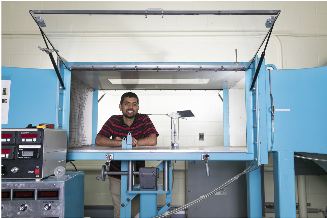
Figure 7.5: Test section of the wind tunnel showing the mounted cyclic pitch turbine and the controllers.
