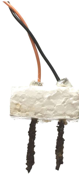
Figure 2-6: Corroded resistive sensor probe
