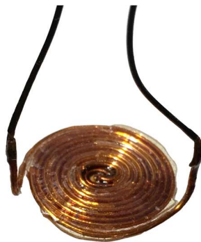
Figure 3-5: Flat bifilar coil, enamel coated wire
