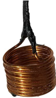
Figure 3-4: Cylindrical bifilar coil, enamel coated wire
