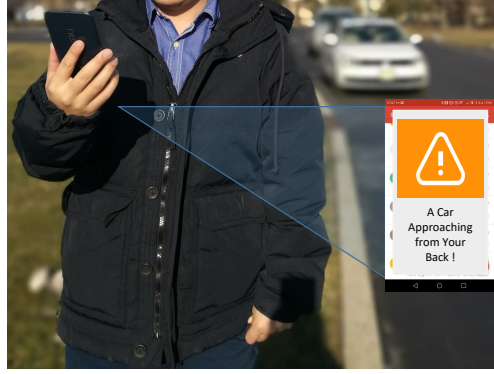
Figure 4.1: Auto++ detects approaching cars using audio data recorded by smartphones. This capability can enable applications such as alerting distracted users (possibly through sounds or vibrations). Please note that the application logic such as alerting users is not part of Auto++ .
