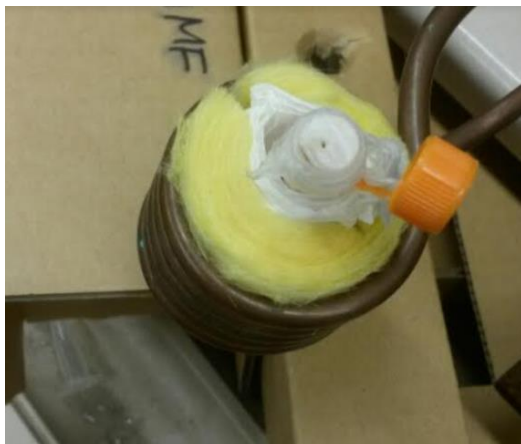
Figure 1: How a sample is placed inside a magnetic hyperthermia coil.
