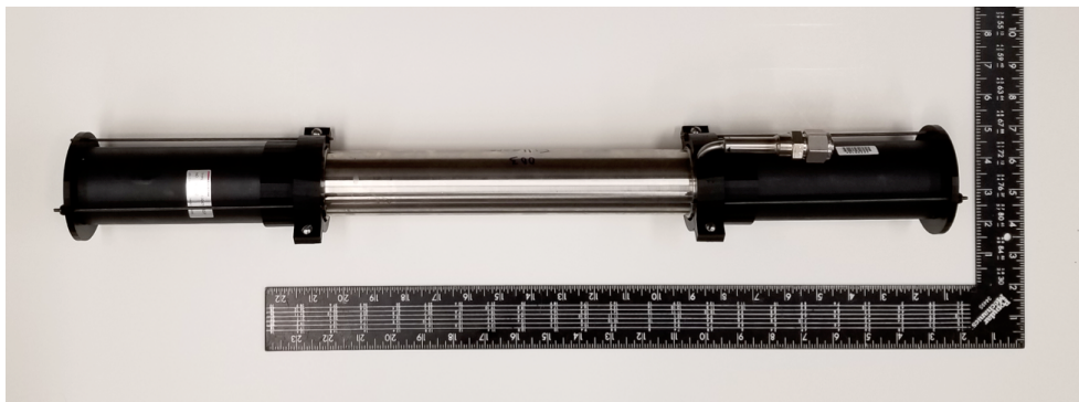
Figure 3.23: SABRE bar type liquid scintillator used for neutron detection in reaction studies.
