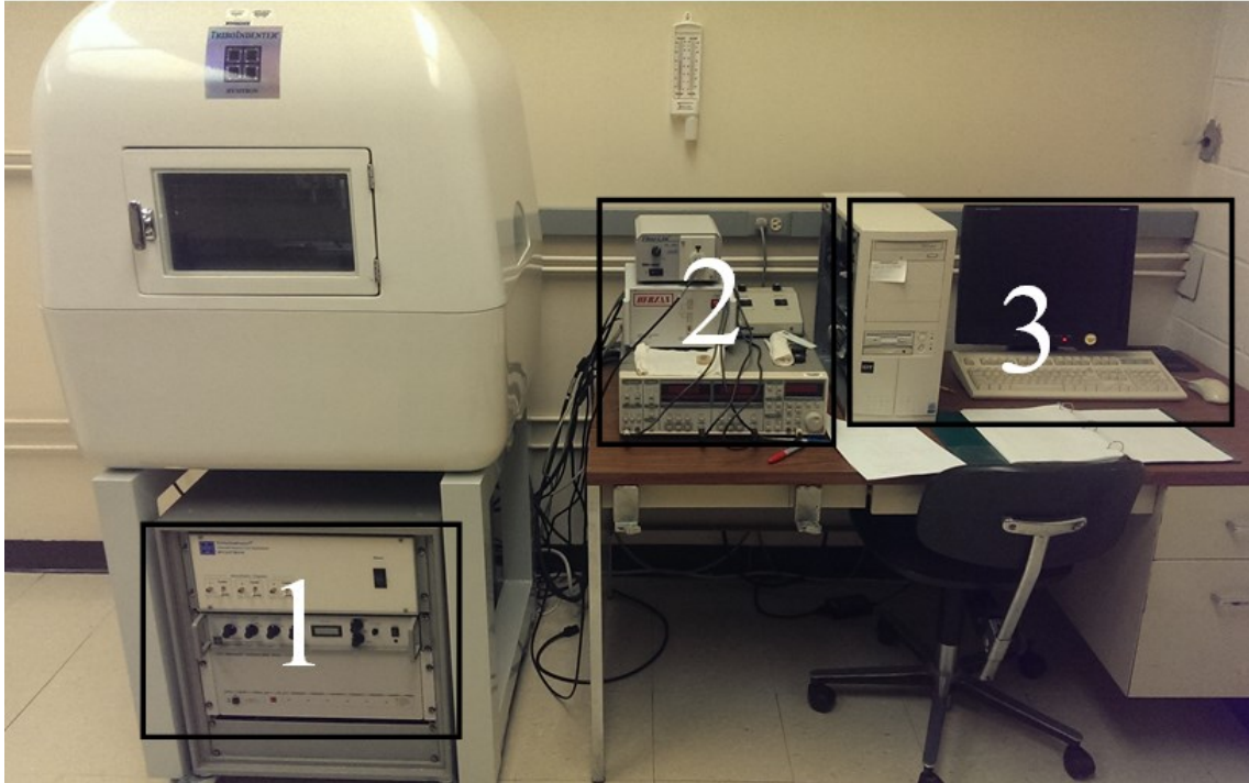
Figure 3.1: The Triboindenter system is shown; it is turned on in the numbered order. The large white “egg” is the chamber in which the tip and sample are located.
