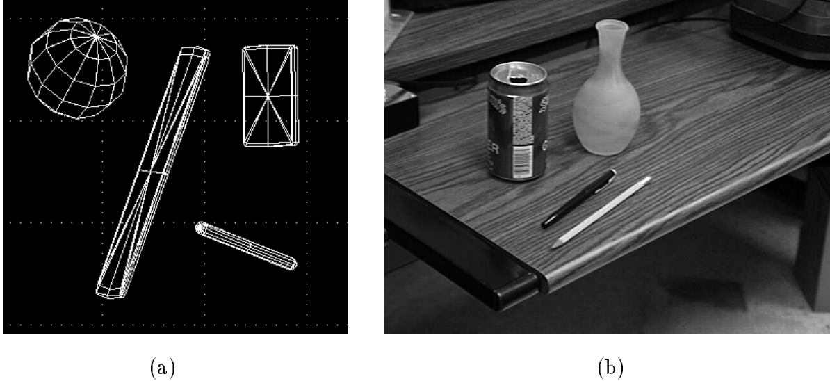
Figure 2: Shape Primitives: (a) The four primitives modeled by superquadrics using Pentland’s Thingworld [20]. (b) Two blobs (can and vase), two sticks (pencil and pen), and a plate (table).
