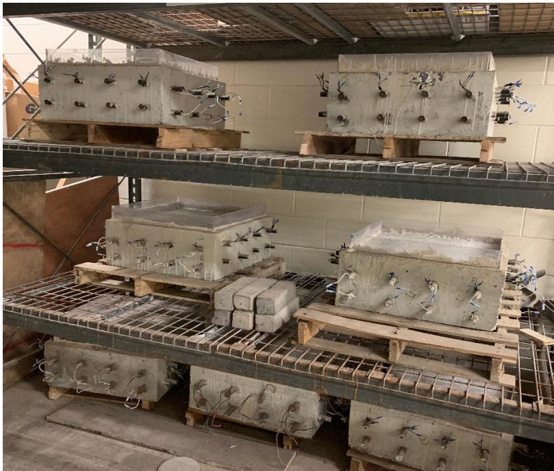
Figure 3–17 Set up of the corrosion slabs
