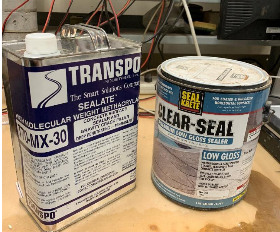
Figure 3–9 Crack sealant that used in this research
