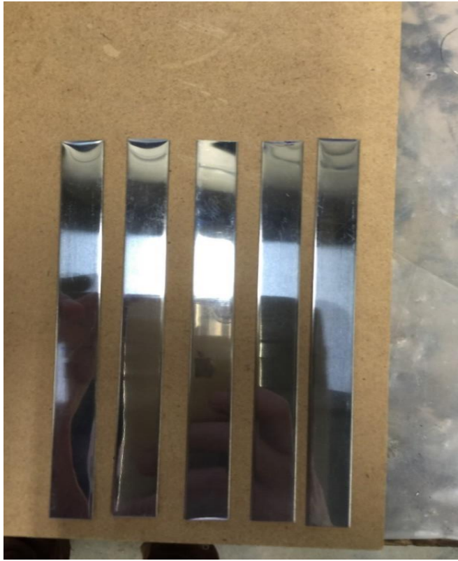
Figure 3–10 Stainless Steel Sheets of the Artificial Crack Formation
