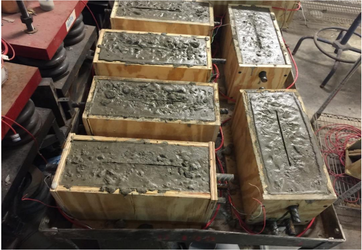
Figure 3-12 The Cracked Concrete Samples after Removing the Stainless Steel Sheets
