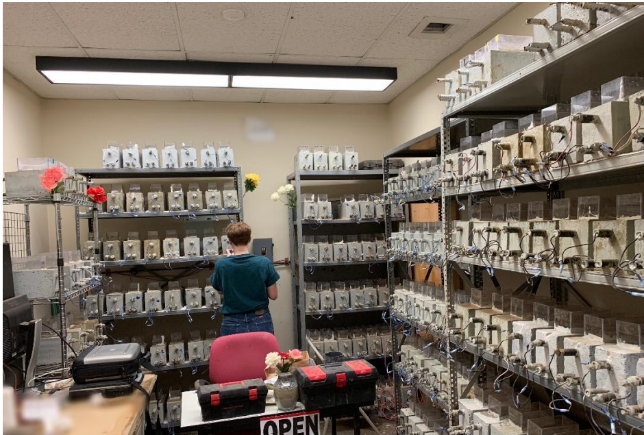
Figure 3–16 Set up of the prismatic corrosion samples
