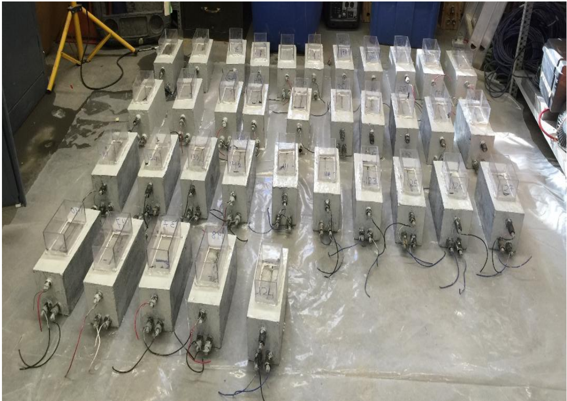
Figure 3–5 Prismatic Samples of Corrosion Tests
