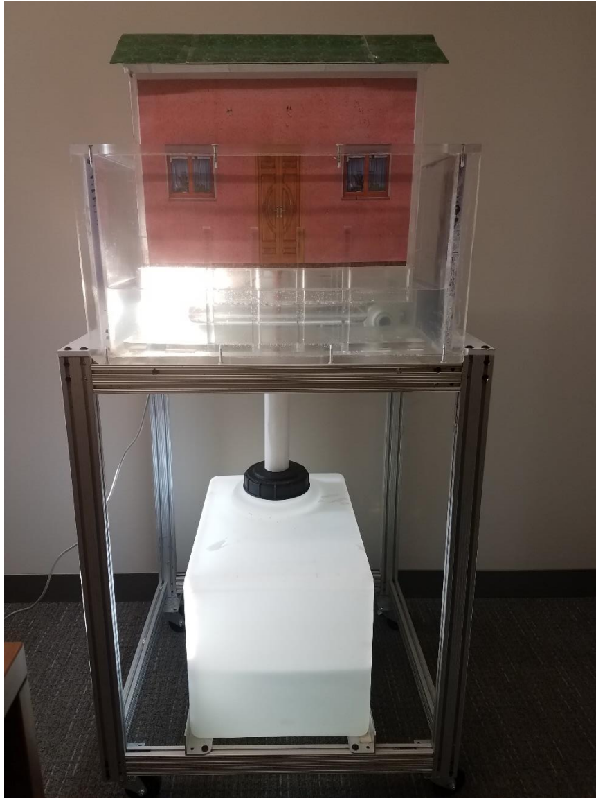
Figure 98. The water continues to rise to the simulated flood level but stays less than the top of the base slab.
