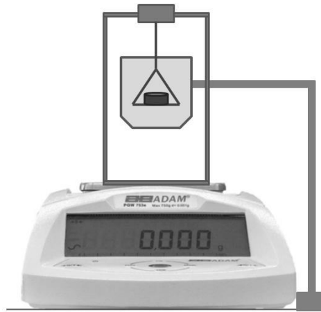
Figure 23. Archimedes density measurement set-up
