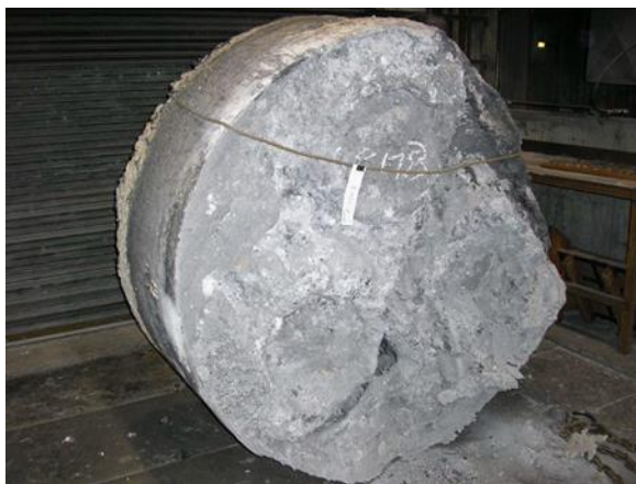
Figure 10. An ingot of boron carbide Sections (a) unreacted material while (b) well-reacted crystalline boron carbide with some possible graphitization [44]
