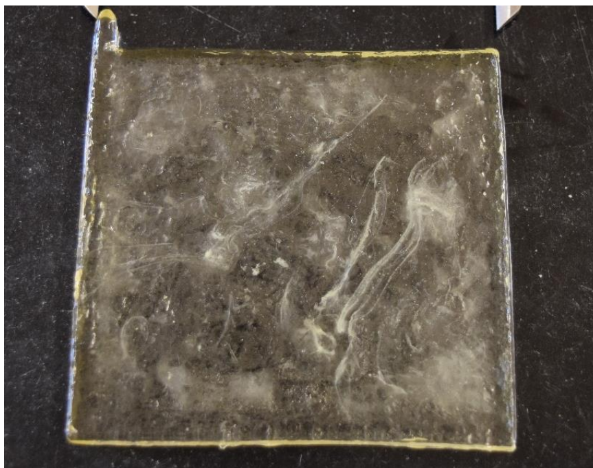
Figure 11: Scaled up piece of Al-35 glass for ballistics impact response tests. Inhomogeneities can be observed in the glass due to the small forming region in this glass family and scaling up the composition.
