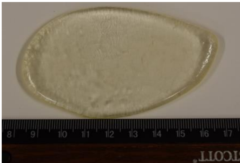
Figure 4: Monolithic piece of Al-35 ( \text{MgO-Y}_2\text{O}_3\text{-Al}_2\text{O}_3\text{-B}_2\text{O}_3 ) as-synthesized after annealing.
