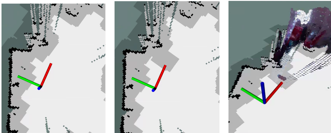
Figure 4.5: Obstacle Detected by the Camera added to the occupancy grid , (toleft) Result without Camera (topright)Result with Camera, (bottom) Voxel Filter imposed on the Occupancy Grid for visualization
