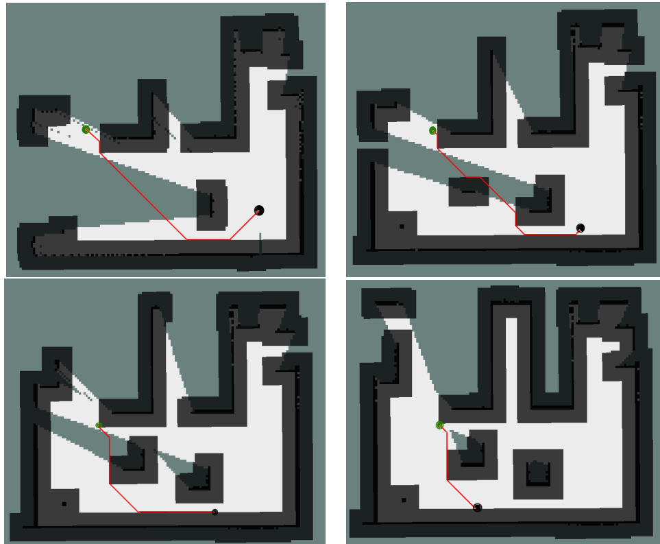
Figure 4.7: The replanning process, the top right figure shows that the planner detects an obstacle on the path and replans the path as seen in the bottom left figure. The bottom right figure shows the result of search of new goal position in the vicinity of the original goal for replanning
