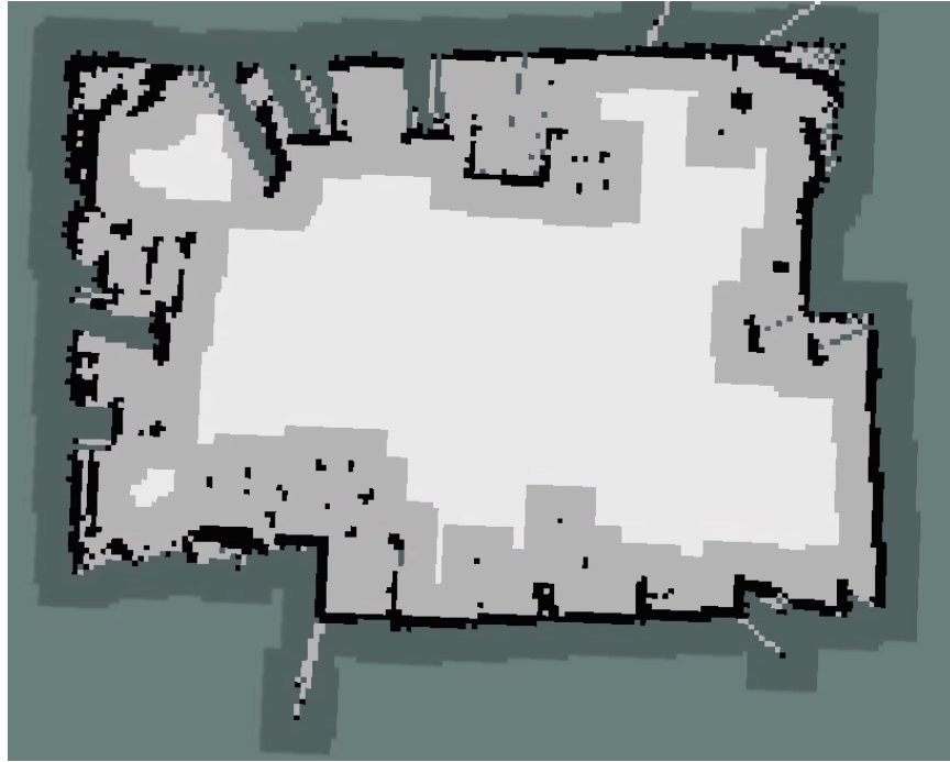
Figure 4.2: Obstacle Inflation Result (White Spaces is the obstacle free space)
