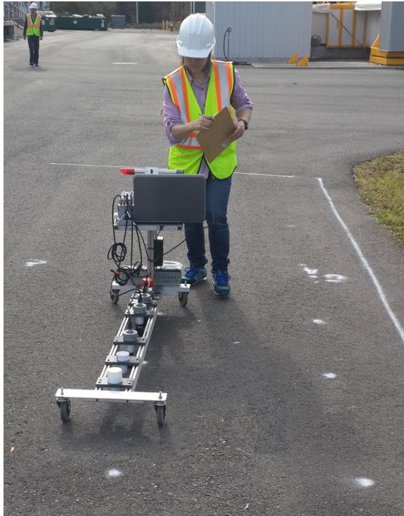
Figure (6-15) Implementing air-coupled SASW testing, case study1
