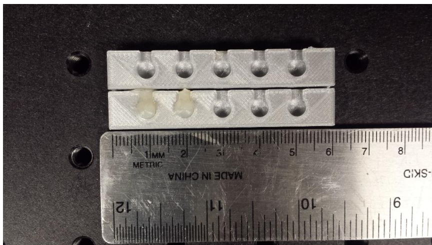
Figure 17: 5 mm diameter agarose inclusions containing Er-doped ReANCs, formed in 3D printed molds.
