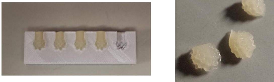
Figure 38: Custom molds (left) were 3D-printed and filled with agarose mixtures to produce inclusions of irregular shape (right).
