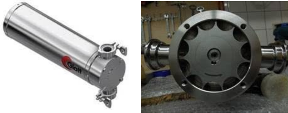
Figure 4-2: Rotary valve external view (left) and internal structure (right).
