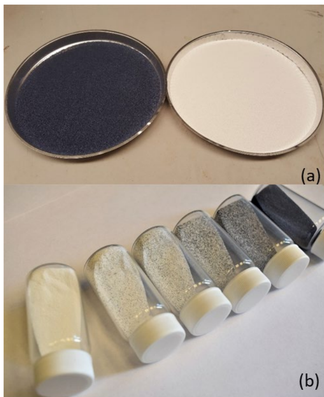
Figure 4-8: Tracer powder. (a) DCPA tracer (left) vs. DCPA powder (right) and (b) DCPA powder mixed with different concentrations of the tracer.
