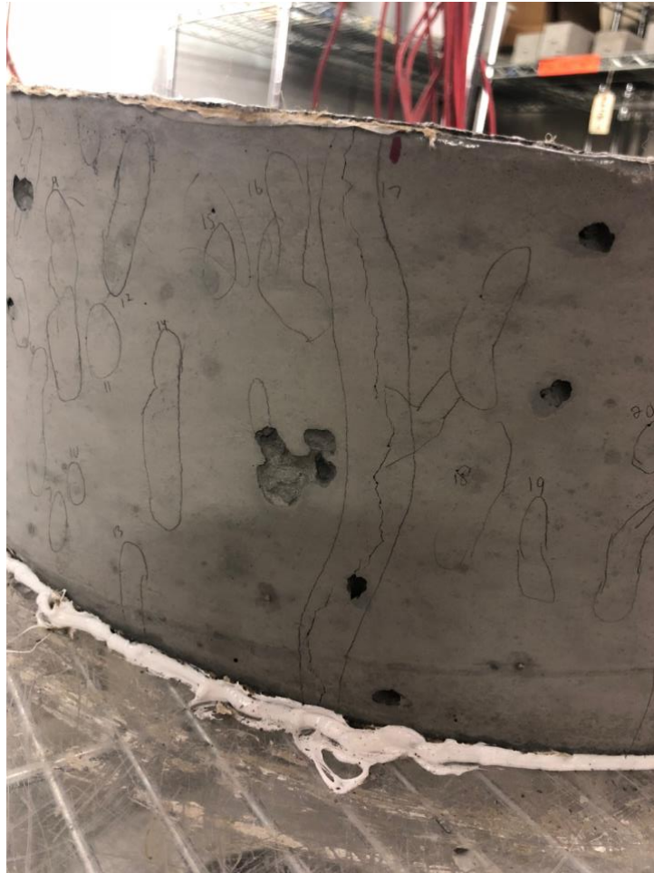
Figure 3.19 – AASHTO ring specimen with a visible full depth macrocrack
