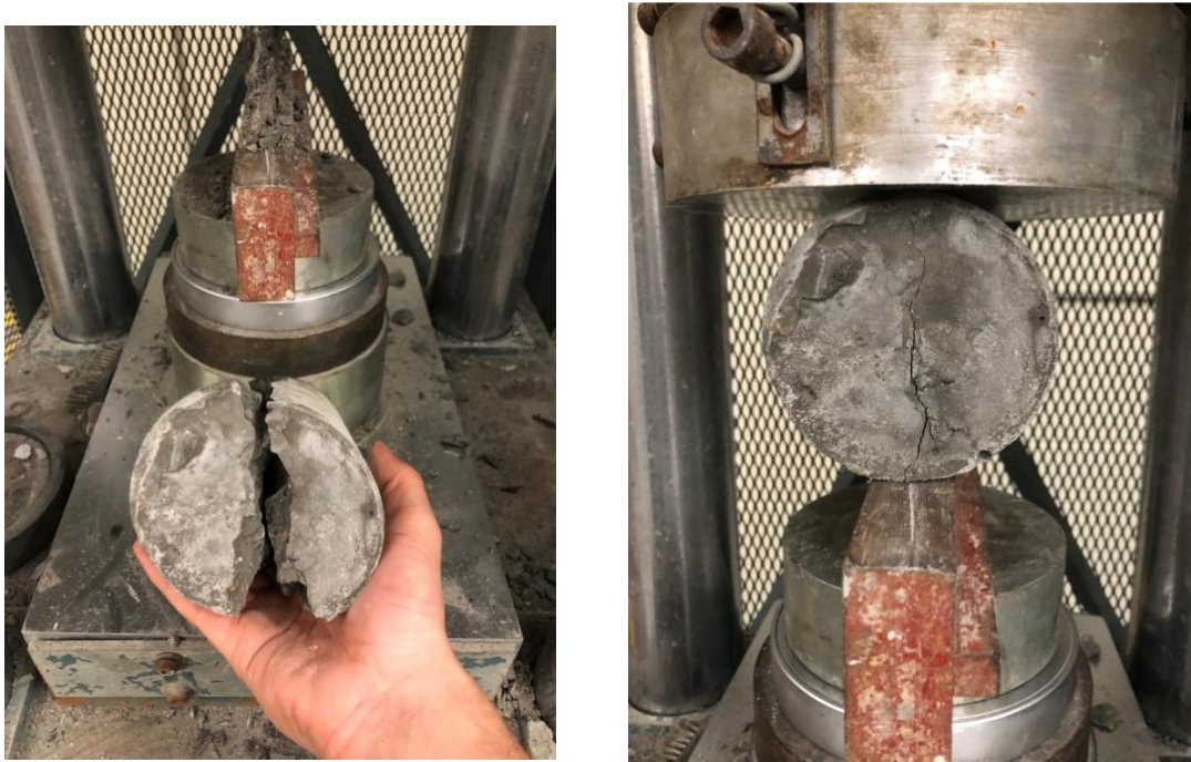
Figure 3.12 – Tensile strength testing of samples with and without fibers
