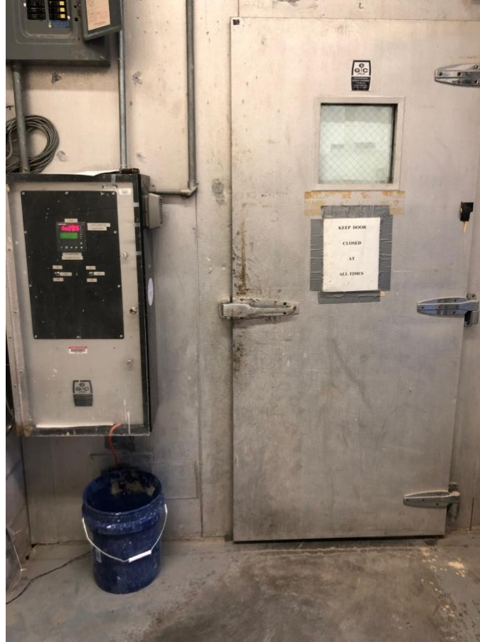
Figure 3.8 – Environmental chamber held at constant temperature of 74° and 50% humidity
