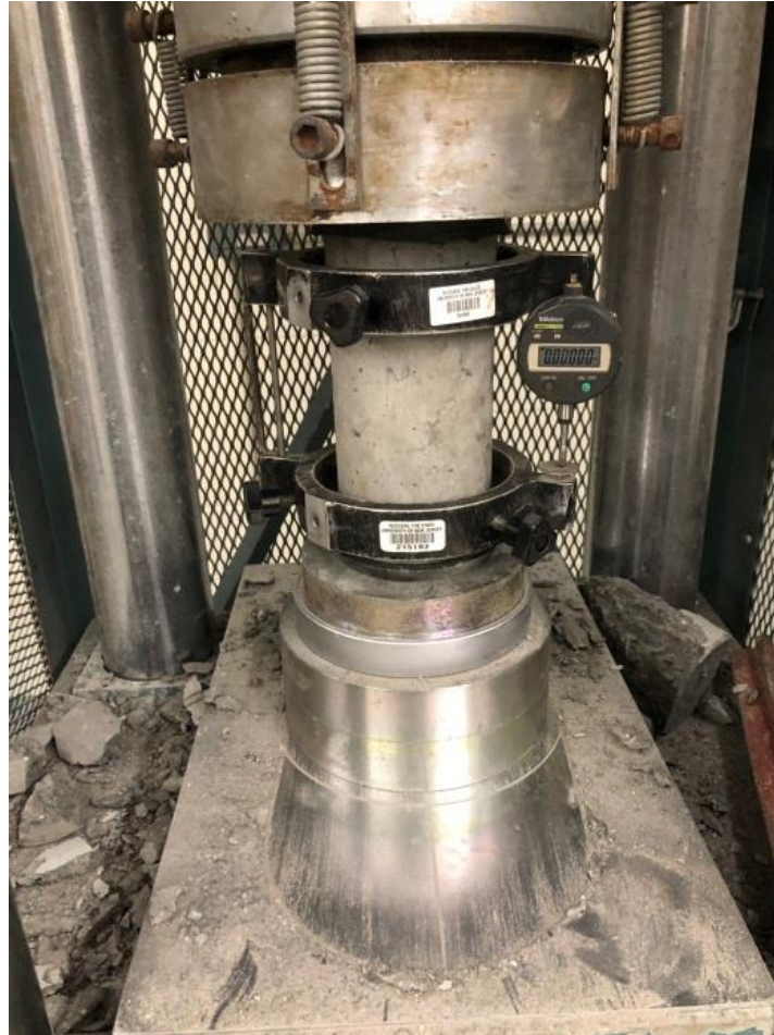
Figure 3.13 – Test sample with modulus cage in testing machine
