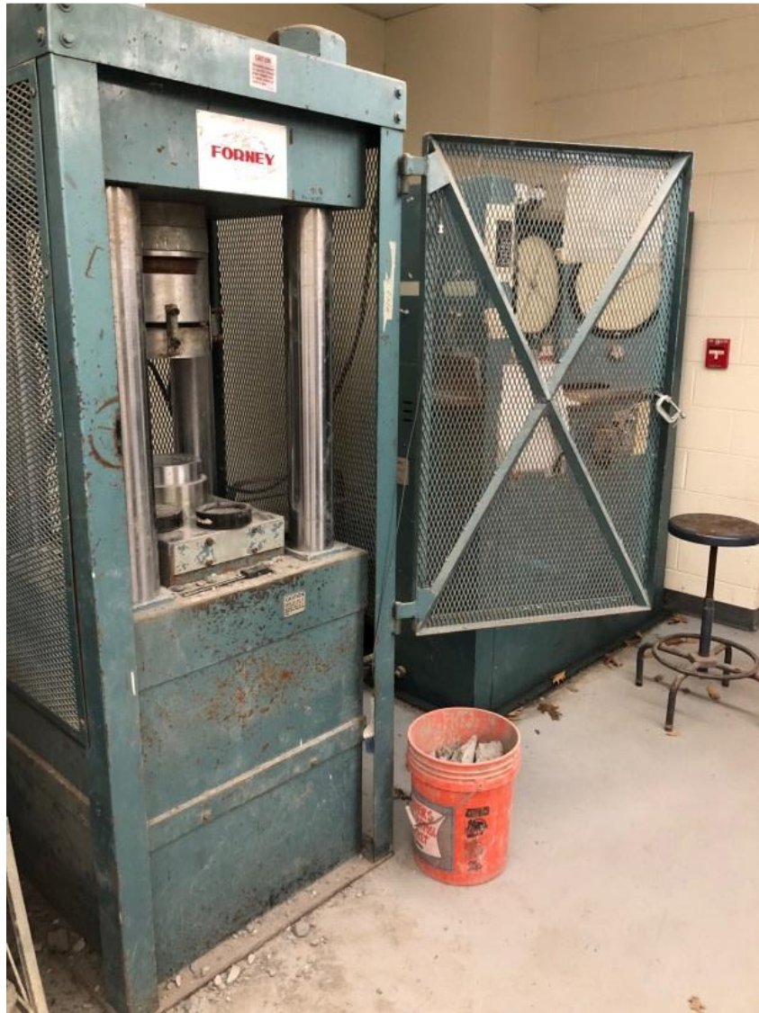
Figure 3.10 – Forney testing machine used to for compression, tension, and elastic modulus tests
