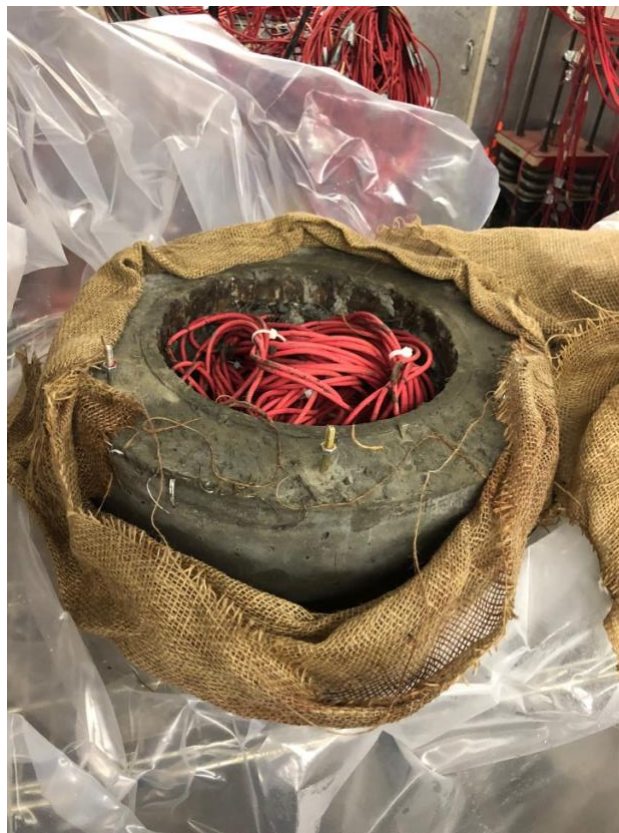
Figure 3.9 – Wet-curing of AASHTO ring specimen
