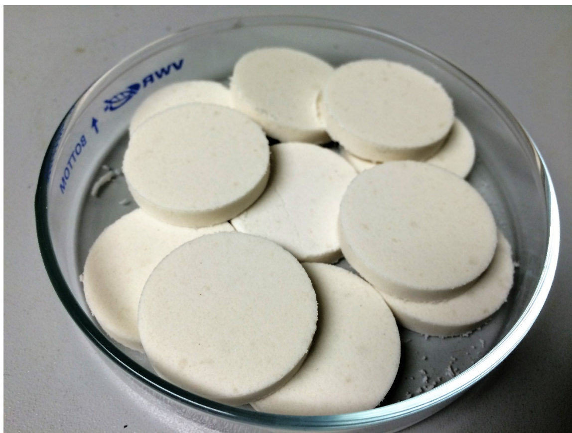
Figure 15. Compacted 7.5% (w/w) canola oil : white rice flour samples.
