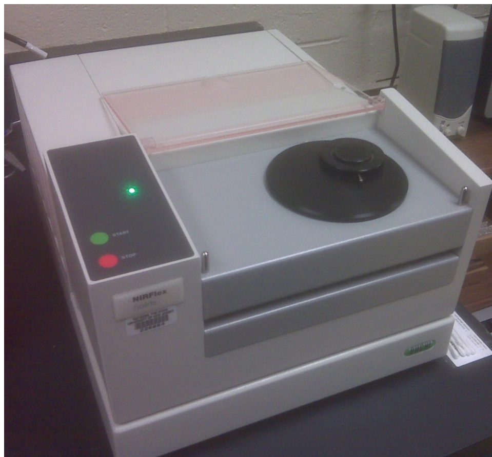
Figure 12. Buchi NIRFlex Solids N500 FT-NIR instrument used in this study.
