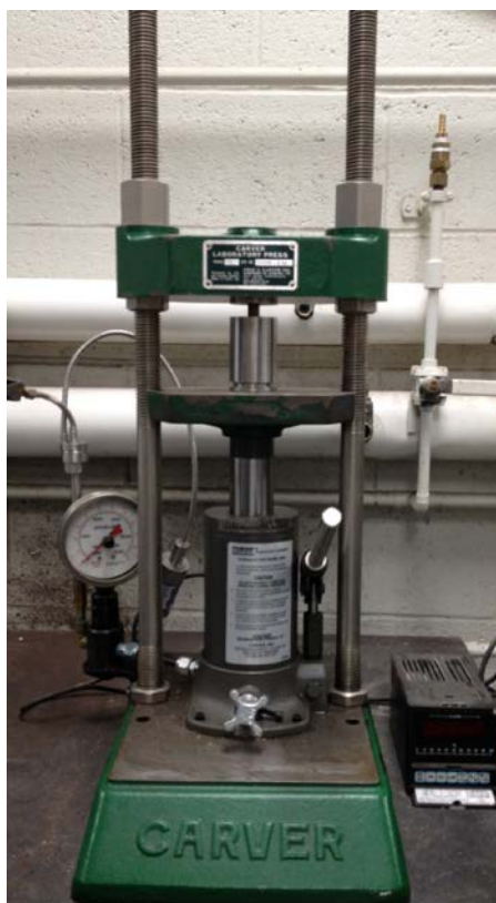
Figure 13. Carver hydraulic press used to prepare sample tablets for NIR analysis.
