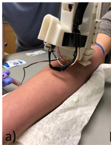
Figure 3: a) Hand-held venipuncture device prototype and setup; b) Results from device use in human pilot study. Average procedure time = 94s. 85% first-stick success rate (11/13). 25G Exel brand needle was used. Skin tone based on Fitzpatrick scale. 12 of 13 patients noted little to no pain during the procedure.
