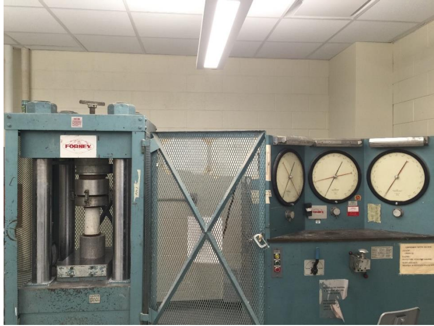
Figure 3.12. 1-Million lbs. Forney Testing Machine
