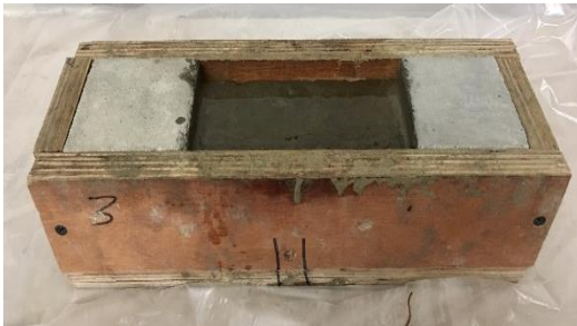
Figure 3.3. Composite Prism: (a) Dry Curing for Six Months, (b) Moist Curing Before Preparing.
