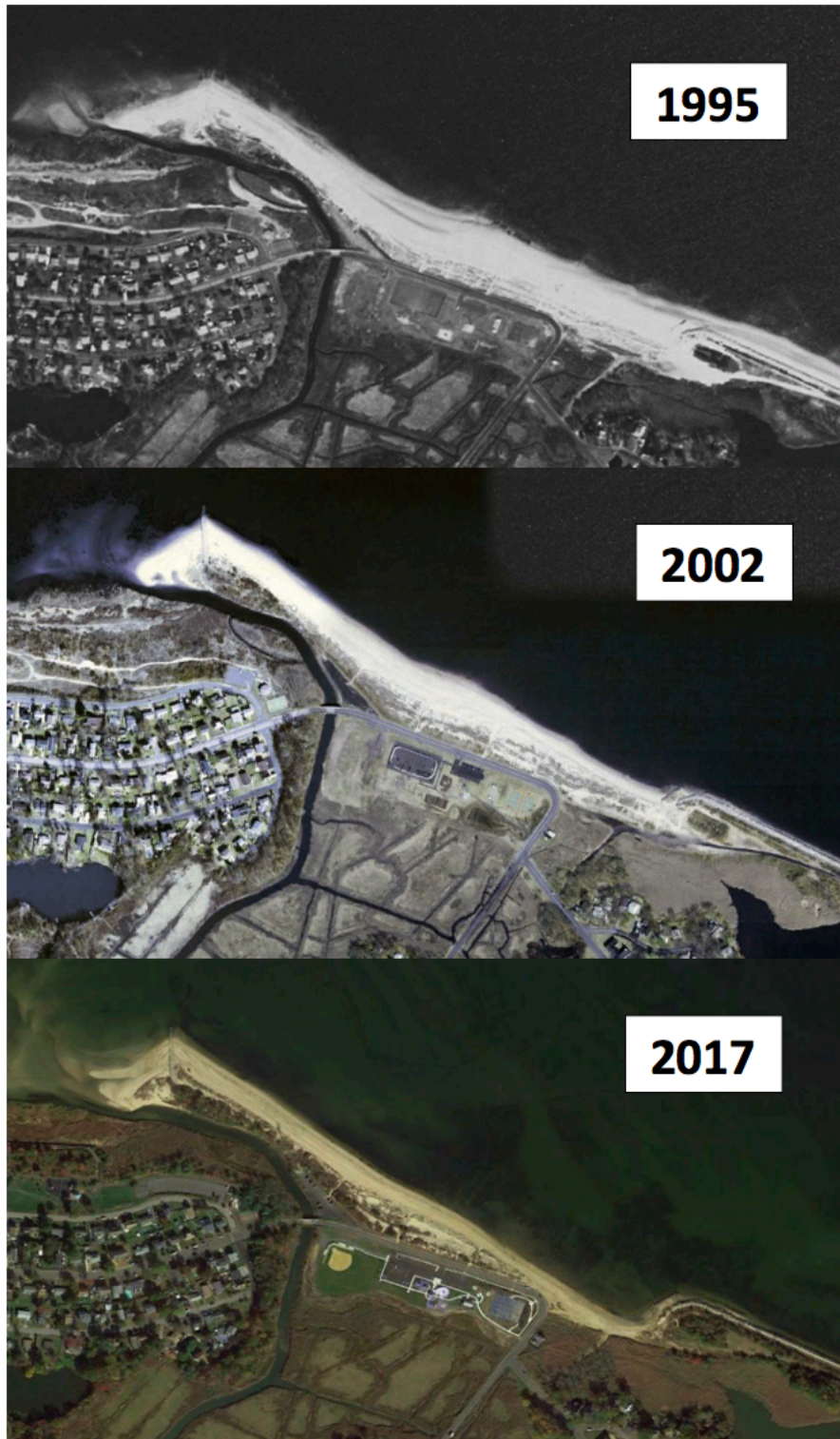
Figure 7: Cliffwood Beach photographs from 1995, 2002, and 2017. 2002 Represents the point in time where all fill sand emplaced in front of the seawall has been transported downdrift into the beach system.
