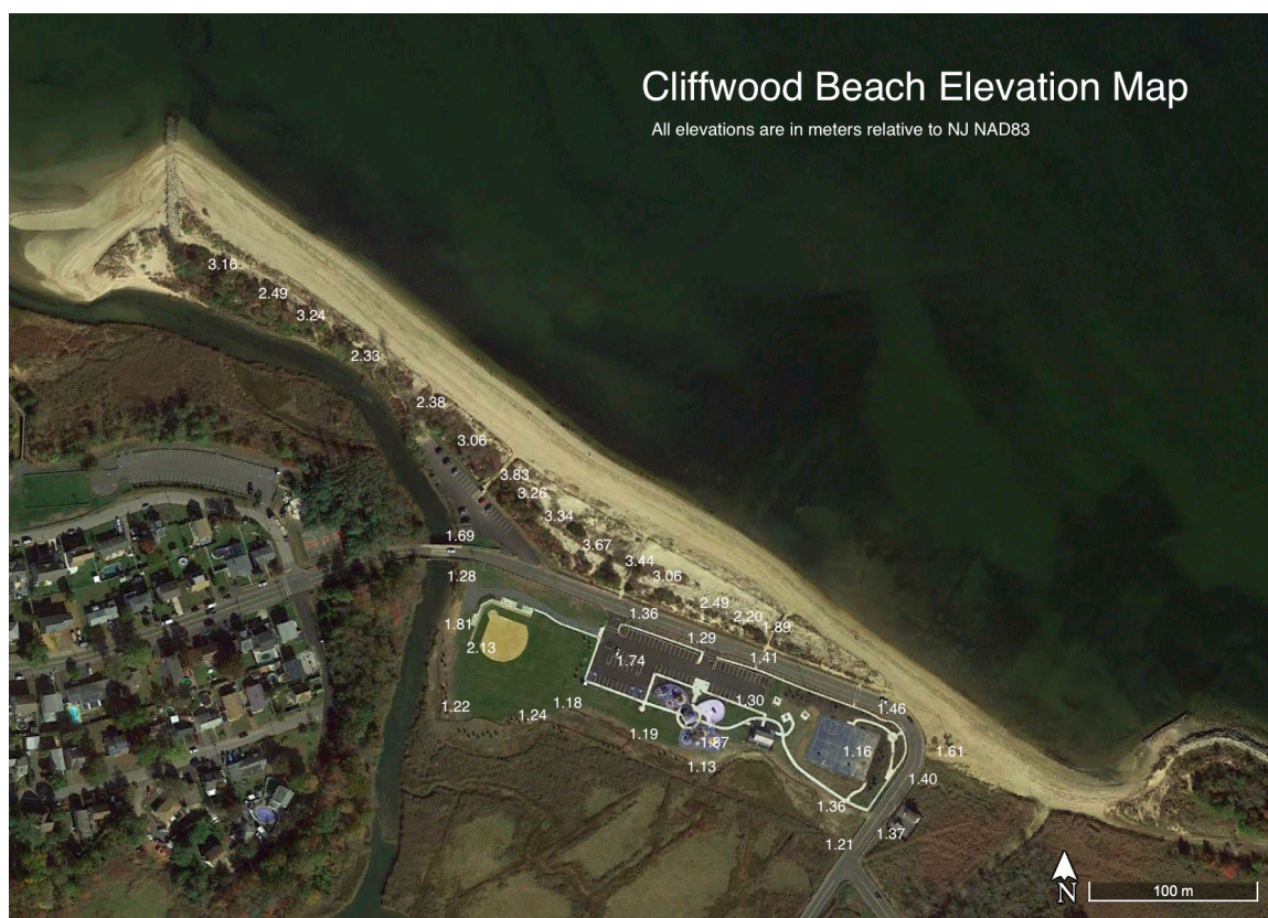
Figure 12: Spot elevations of high and low points in the dune system and surrounding areas. All elevations are in meters, relative to NJ NAD83.
