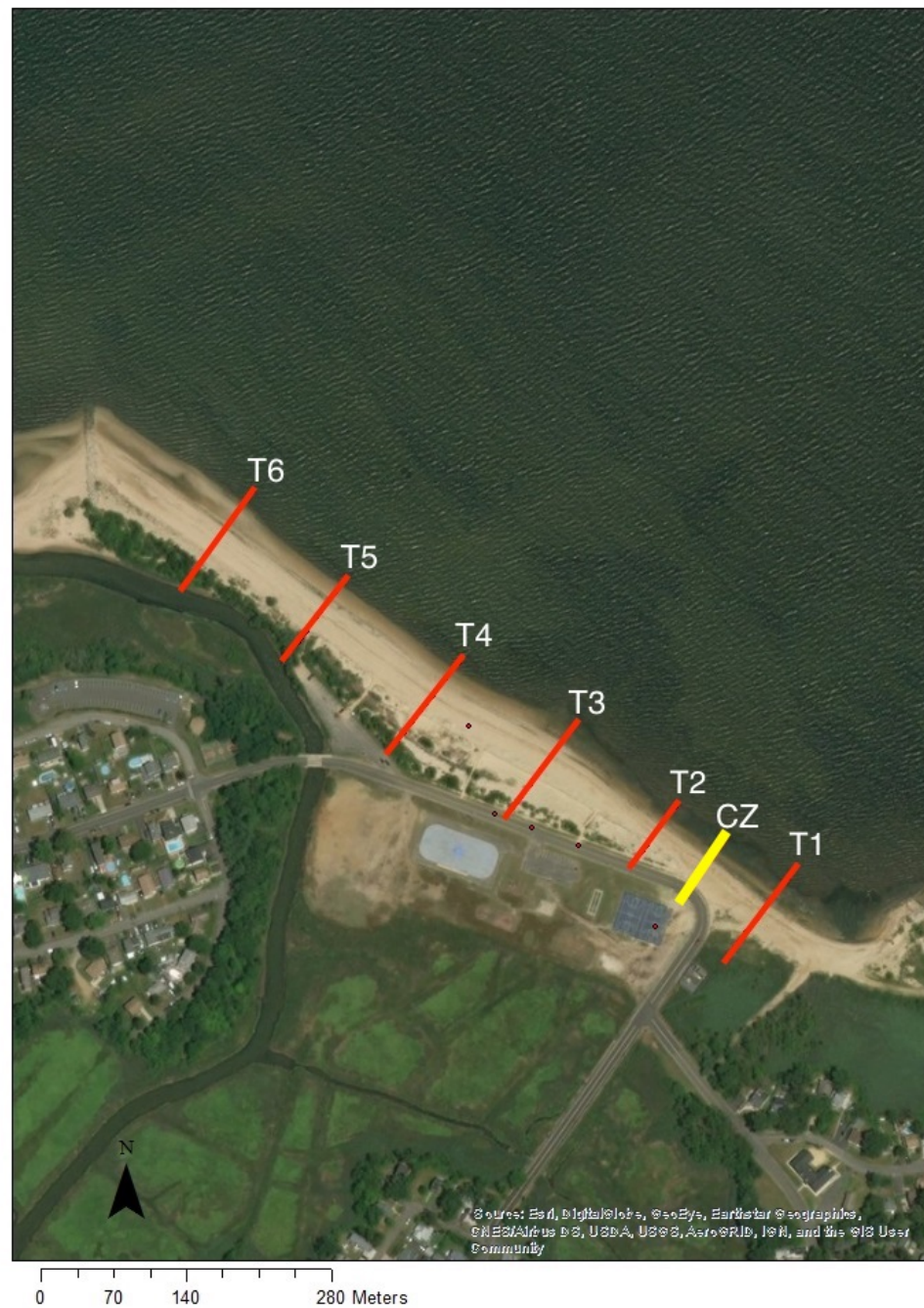
Figure 5: Map showing the location of the six numbered transects monitored every three months December 2017-December 2018 using an RTK GPS unit. Profiles at CZ were taken only in December of 2017.
