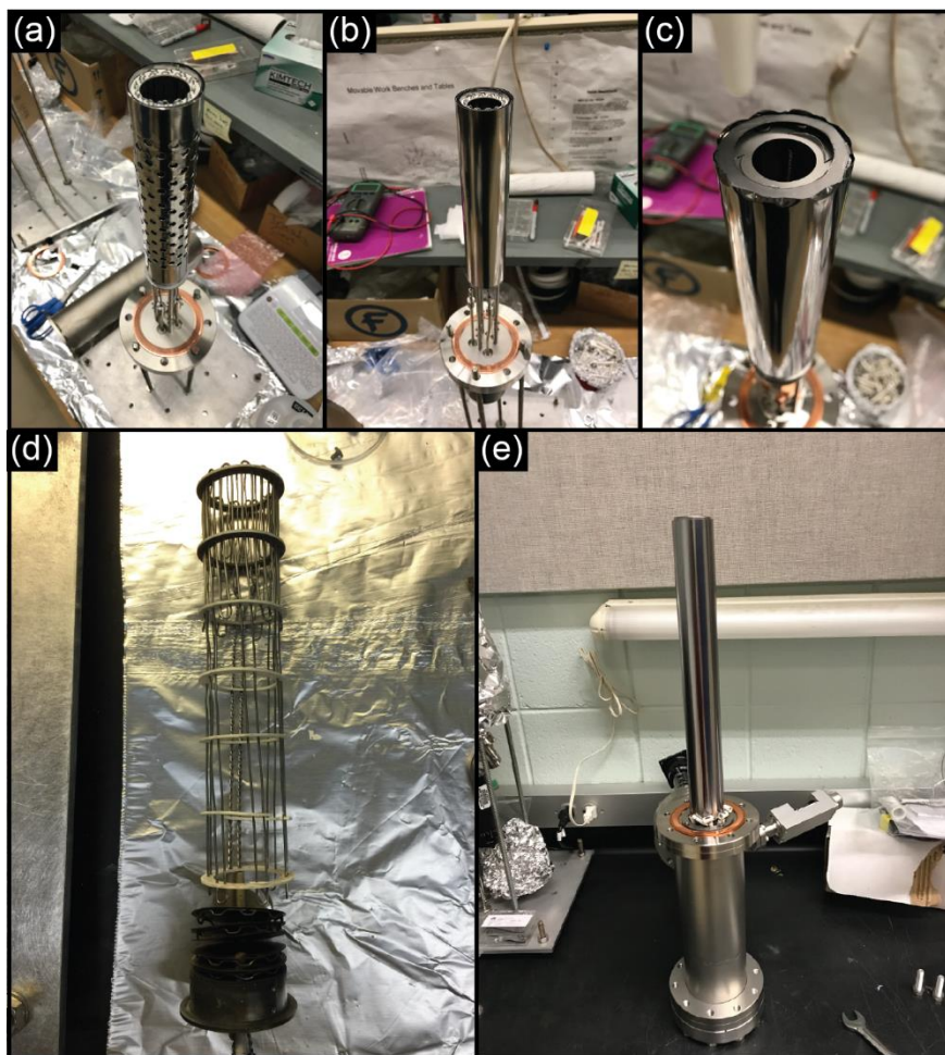
Figure 2-8. Pictures of thermal effusion cells. (a) Low-, (b) Medium-, (c) High-temperature thermal effusion cells. (d) Inside coil of an effusion cell. (e) Se cracker cell.
