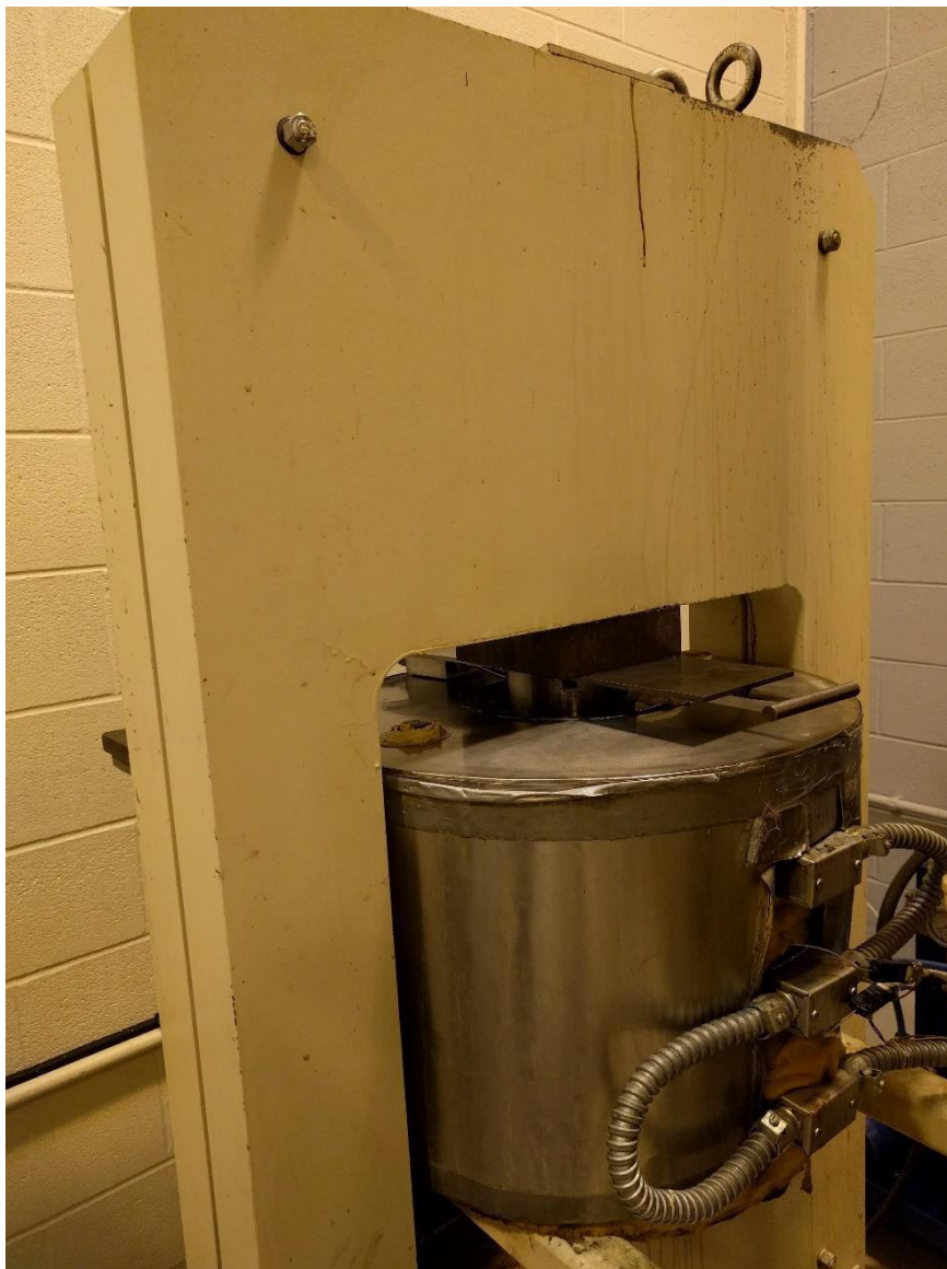
Figure 18: 1.5 L High Pressure Processing vessel at Washington State University, Pullman, WA.
