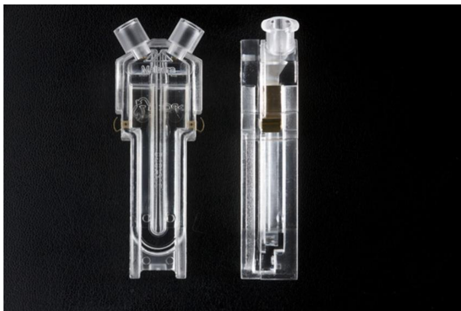
Figure 28: Folded Capillary cell used to measure zeta potential.
