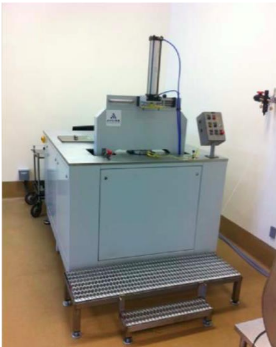
Figure 20: 2 Liter HPP unit at University of California, Davis.
