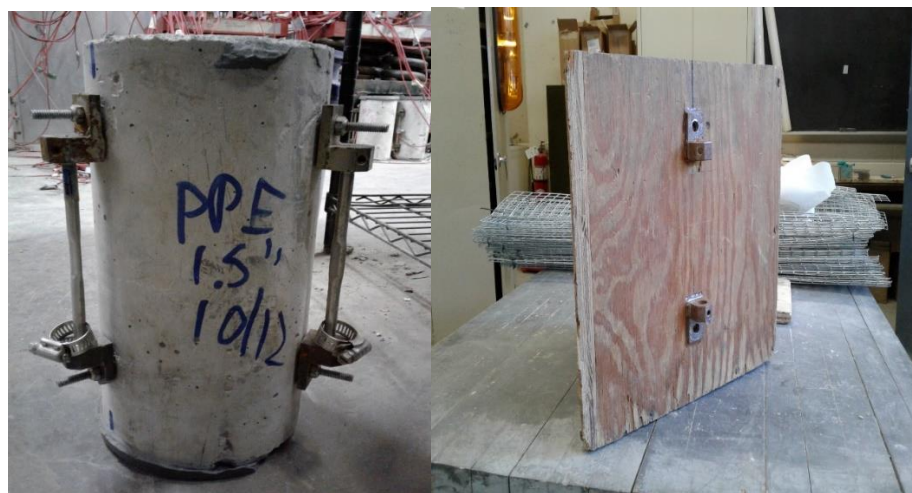
Figure 3-24: Vibrating Wire Strain Gages on the Side of a Concrete Specimen
