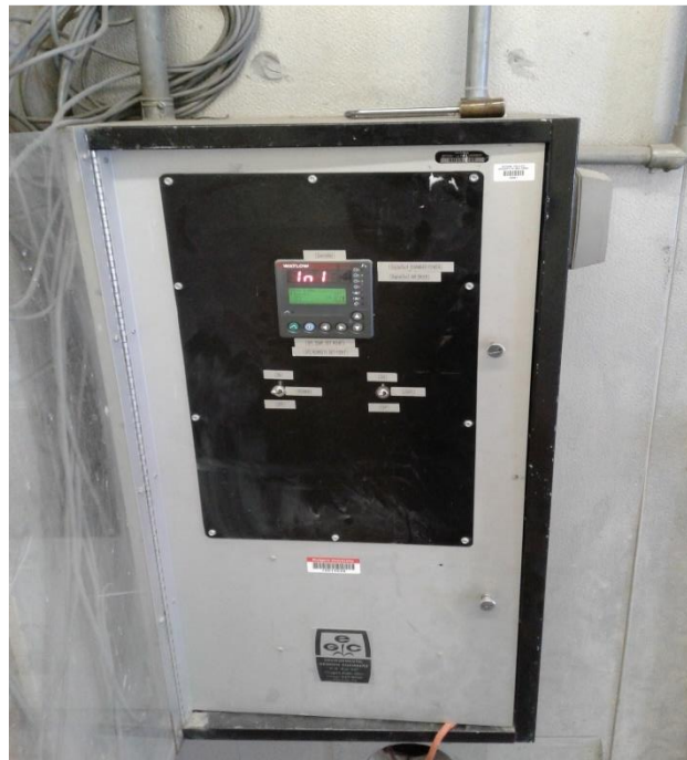
Figure 3-19: Digital Control Unit for Environmental Chamber
