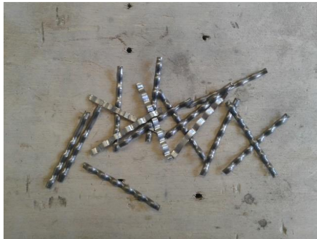
Figure 3-2: Steel Fibers, Crimped Shaped and 1.5'' Length
