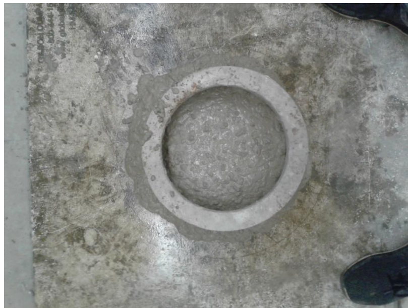
Figure 3-6: SCC Slump Flow on the Board
