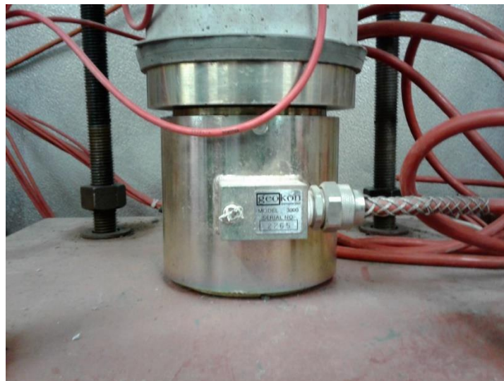
Figure 3-22: Geokon Load Cell Monitoring Load of Rig
