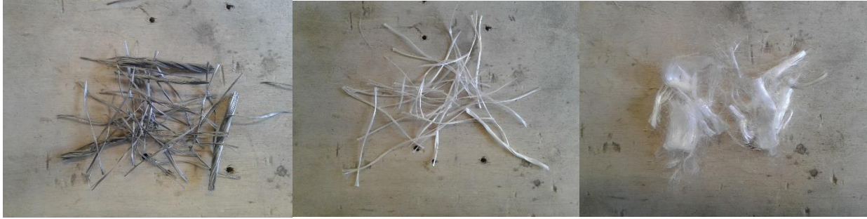
Figure 3-1: Polypropylene Fibers of Length 1.5'', 2.0'', and 0.75''
