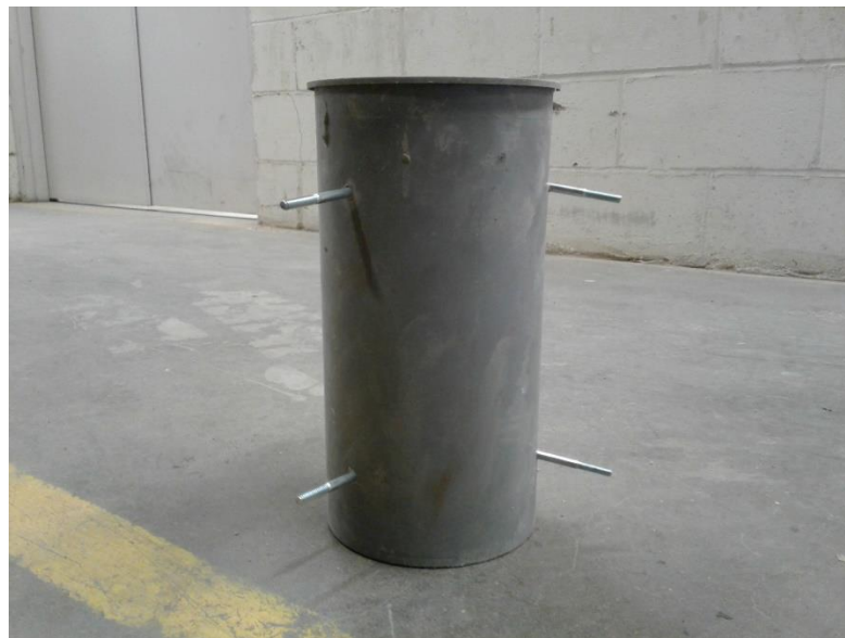
Figure 3-3: 6'' x 12'' Cylinder Modified for Creep Testing
