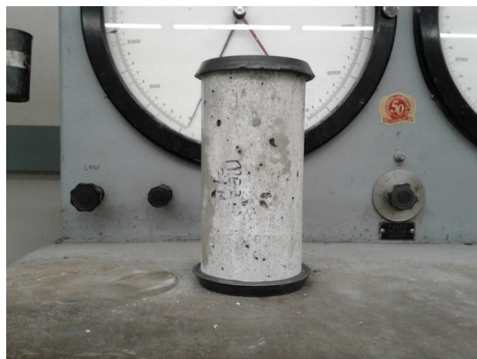
Figure 3-13: Steel Caps on the Concrete Specimens
