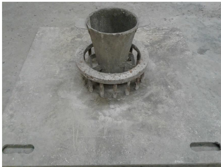
Figure 3-7: SCC J-Ring Test Set Up
