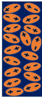
Figure 2. 1. (A) The dipoles are randomly oriented in the dielectric material in the natural state. (B) All the dipoles aligned in the same direction under the influence of an external electric field.
