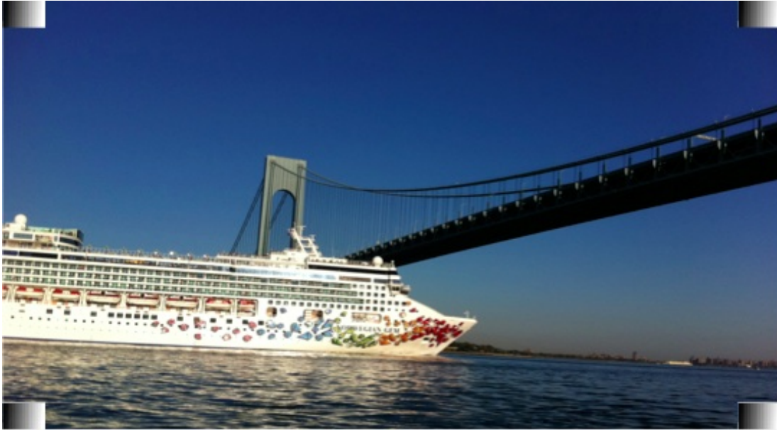
Figure 2.8: Radiometric calibration texture patches (ratex patches). Ratex patches placed in corners and used for radiometric calibration and classification training. Source: [2].
