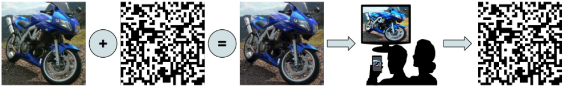
Figure 4.1: Goal of LFM (Light Field Messaging): embed a message within an image or video, display the image/video on-screen, photograph it with a handheld camera, and recover the hidden message. LFM significantly outperforms other synchronization-free steganography techniques for camera-display messaging in message bit recovery error (BER). Source: [4]. Our code and dataset are available here [75].
