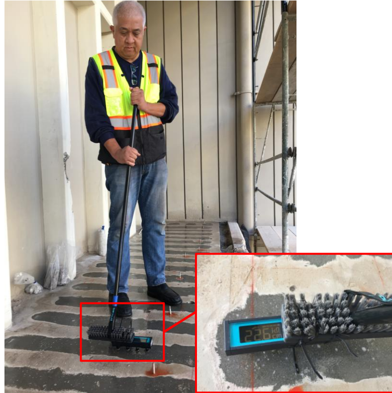
Figure 2-12. Electrical Resistivity measurements using a Wenner probe.
