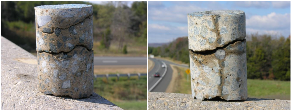
Figure 2-5. Delamination in cores extracted from a bridge deck in Virginia.
