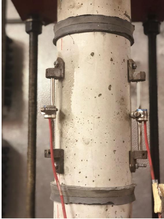
Figure 3-18: VWSG Attached to the 6 x 12 Cylinders
