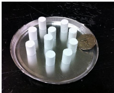
(c) Pellets or pseudo-granules developed were compressed at constant force for a constant time
