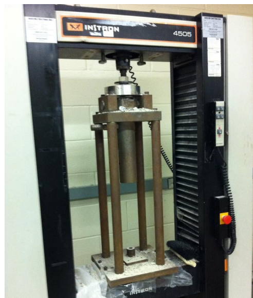
(b) INSTRON Dynamite load frame used to measure stress vs. strain relationship
