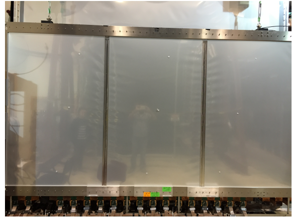
Figure 3.38: Gas gain measurements performed with DC3m ( \text{ArCO}_2 gas). The ^{55}\text{Fe} source is taped on different locations on the drift chamber in order to measure the pulse height.
