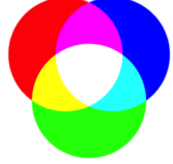
Figure 2.5: Combination of red, blue and green making the overlap region “colorless”
