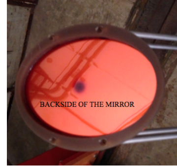
Figure 3.8: Degraded backside of the Čerenkov counter mirror.
