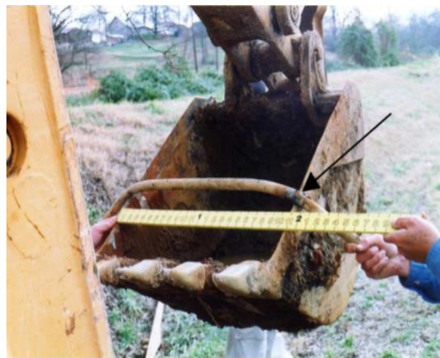
Figure 6: Damaged section of the gas service line NTSB
