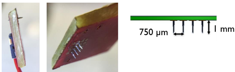
Figure 4.9 (left) 2 nd gen. EP chip pictures with the needles attached. (right) The space between the needles and their protruding length are shown schematically.
