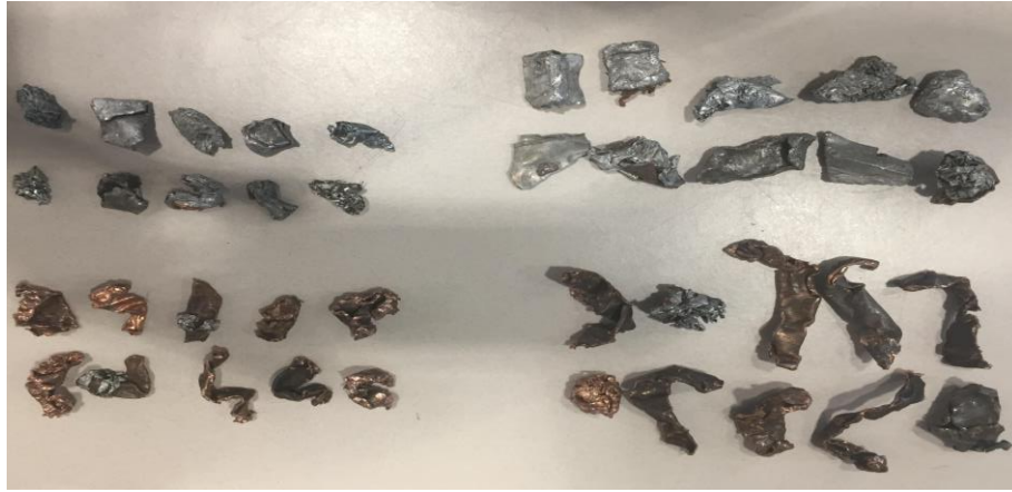
Fig. 36. Test Samples: 10 big / 10 small of copper and aluminum (one set of two used).
