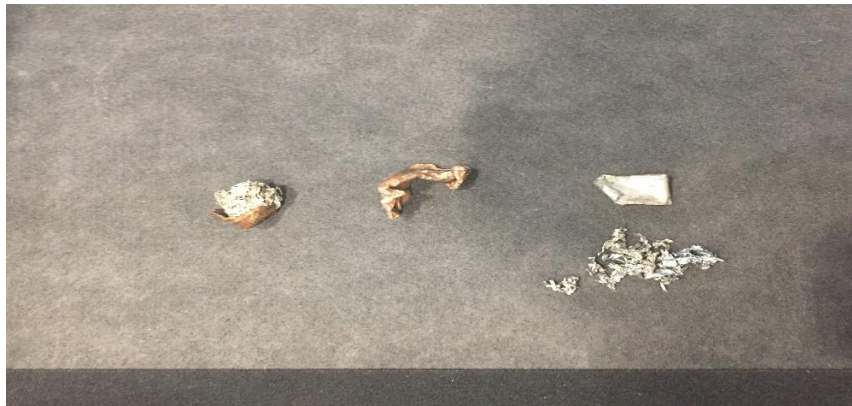
Fig. 1. Sample Pieces for Experimentation: from right to left, piece of pure aluminum, aluminum shavings, pure copper, and mixture of aluminum and copper on conveyor belt.
