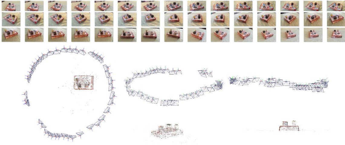
Figure 3-20 Reconstructed point cloud from SfM and camera poses
