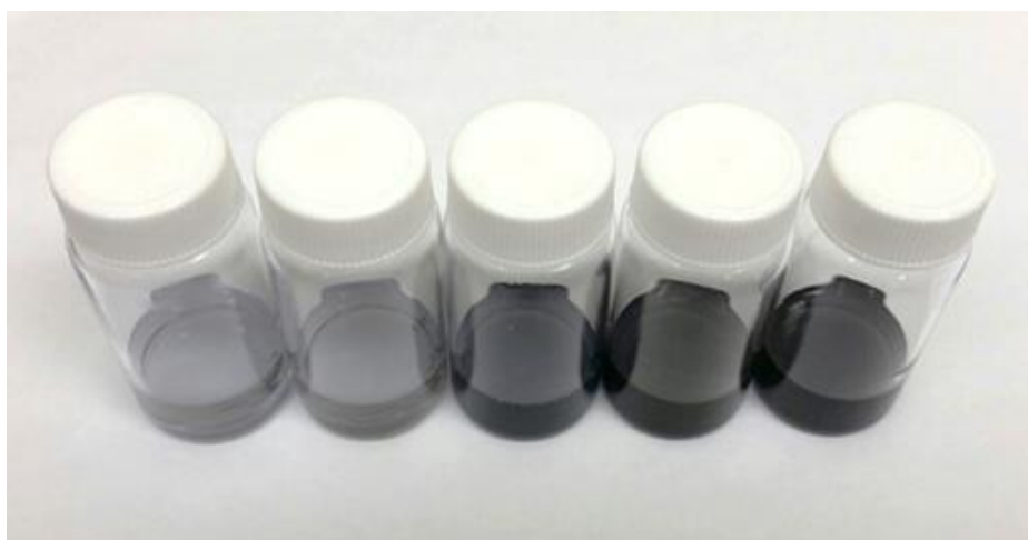
Figure 18: 65%MTES- 35%DMDDES melting gels with Au-nps concentrations from left to right 8,10,12,14,18nM
