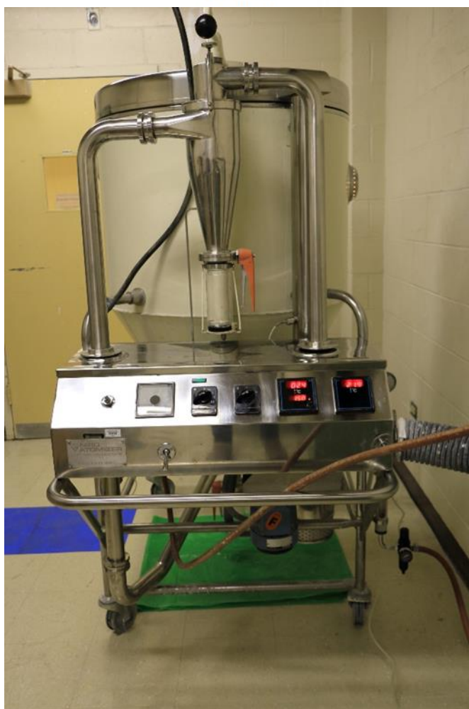
Figure 21. (Top) Schematic drawing of the Niro Atomizer Laboratory Minor Plant and (Bottom) the actual Niro Atomizer used for this dissertation.
