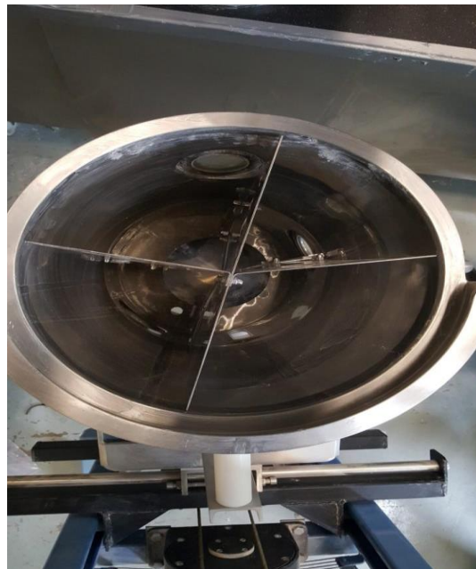
Figure 6-3 Insert of Continuous Fluidized Bed (GCG-2) with four sections
