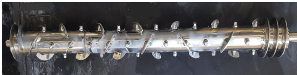
Figure 2-8 Granulation shaft and its blades
