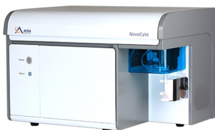
Figure 1.2: NovoCyte Benchtop Flow Cytometer by ACEA Biosciences [5]
