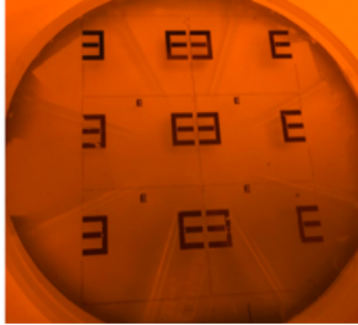
Figure 4.6: Image of fabricated wafer with 12 co-planar electrodes
