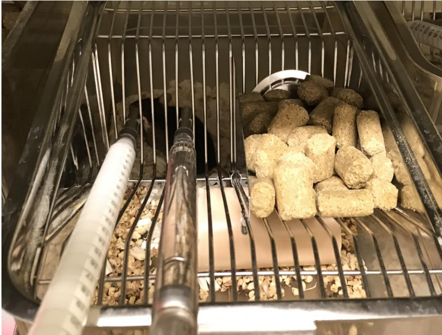
Figure 1: Two-bottle taste preference testing apparatus. Standard home cage wire lid is adapted to fit two volumetric bottles, in addition to ad libitum chow. Left bottle contains lipid emulsion, right bottle contains water.
