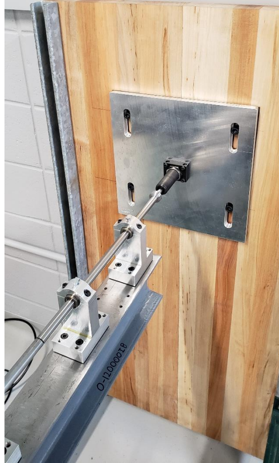
Figure 3.18: The momentum trap consists of a bar and shock absorber.
