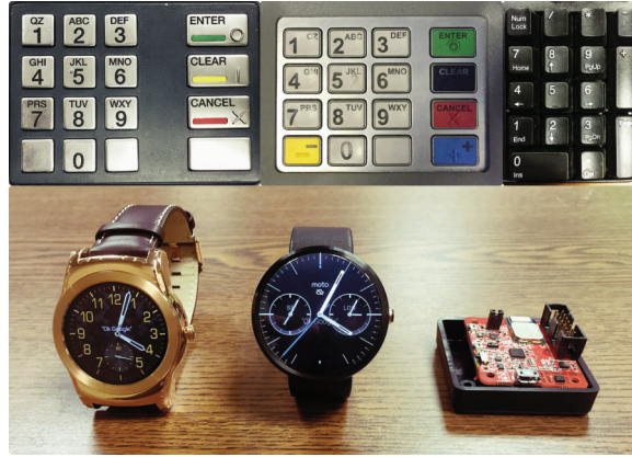
Figure 3.11: Experiments: three different kinds of keypads, detachable ATM pad, keypad on ATM machine, keyboard; and wearable devices.
