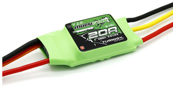
Figure 5.4: Turnigy MultiStar 20A ESC.
