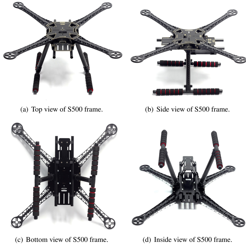
Figure 5.2: S500 quadrotor frame.
