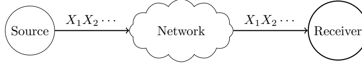
Figure 1.2: The simplest one-to-one active status updating model. X_i indicates the i -th update by the source.
