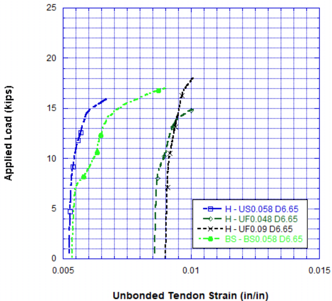
Figure 4.20 Effect of the area of the unbonded tendons at the same depth on the load-strain behavior of the top tendon strain
