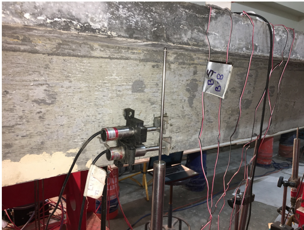
Figure 4.9 Hybrid beam showing LVDT's at mid-span profile for strain profile measurement
