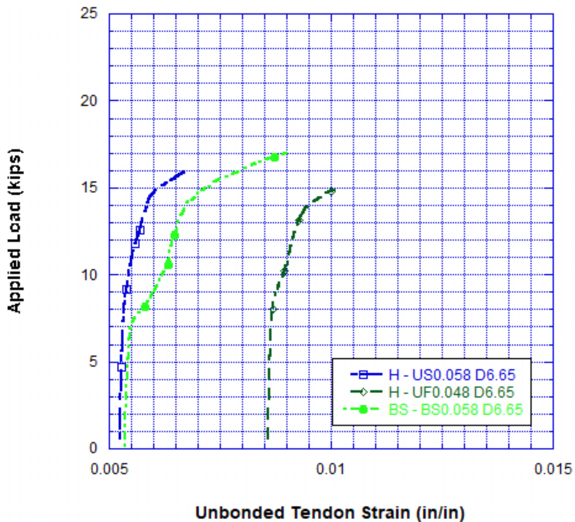
Figure 4.19 Load-strain behavior of the top tendon strain for the hybrid combination compared to fully bonded steel tendons
