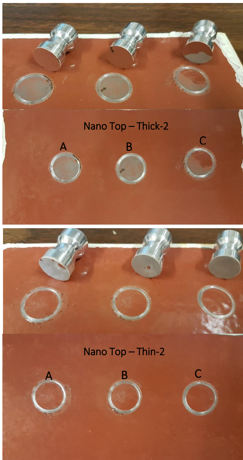
Figure 3-13 Pull off test performed after two month, Batch-3.
