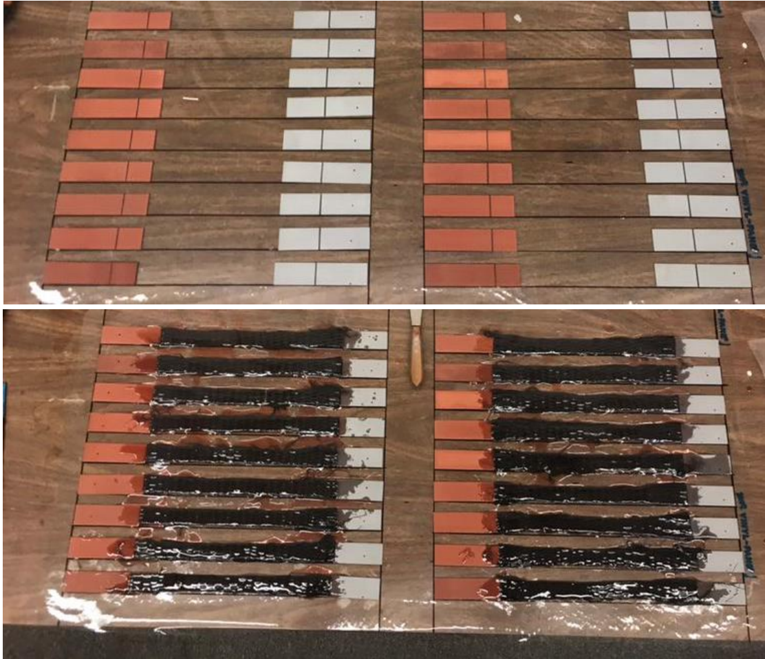
Figure 5-1 Specimen fabrication. Alignment and mark ups pf specimens where black lines show the extend of overlap on both ends of the specimen (top), laying CFRP in place (bottom).
