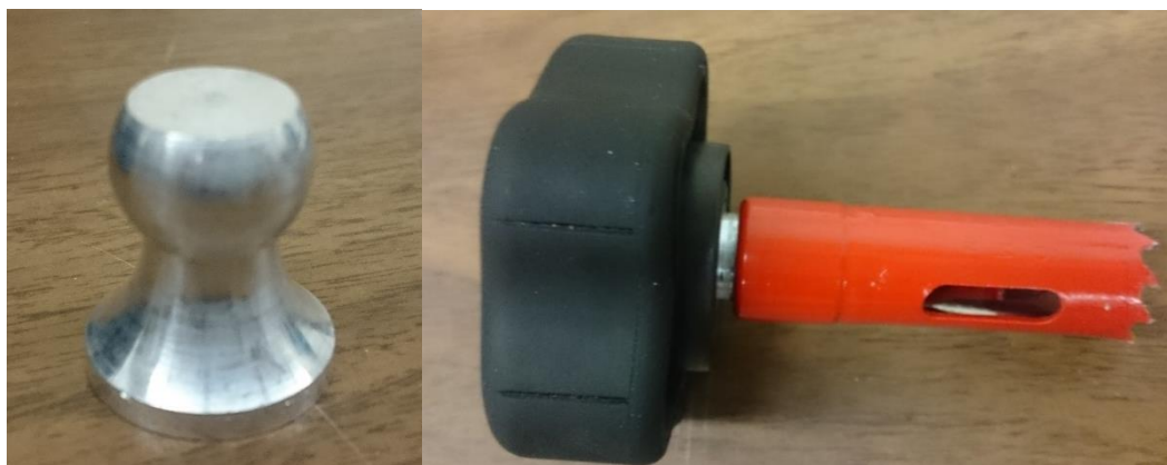
Figure 3-6 Pull off dolly (left), Cutting tool for isolating dolly (right).
