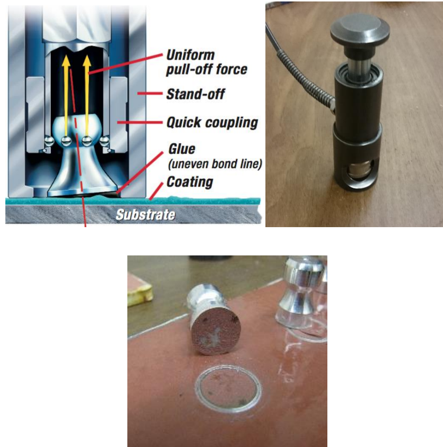
Figure 3-7 Dolly grip (top right) and its schematics (top left), and dolly after failure (bottom).
