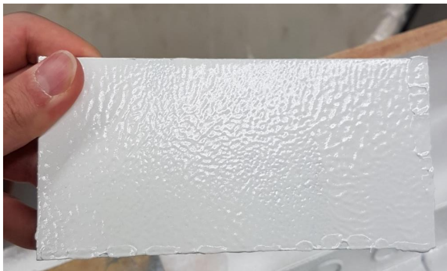
Figure 3-17 Back of a specimen coated with organic coating
