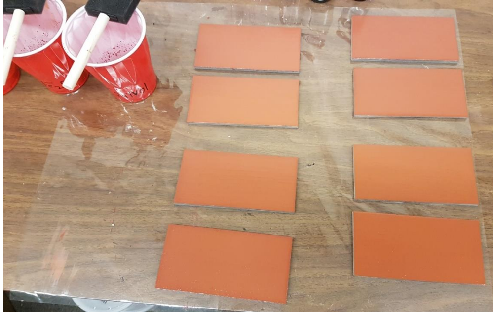
Figure 3-15 Freshly coated specimens using foam brush.
