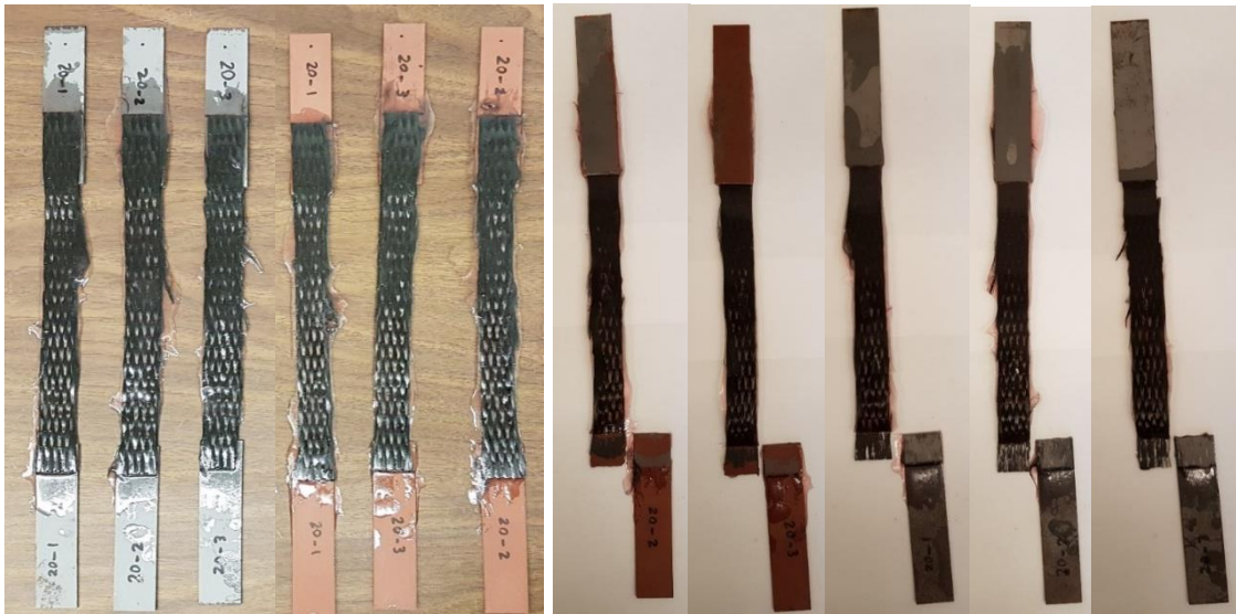
Figure 4-9 Modified Lap-Shear specimens before tension test (left), Specimens after Failure from left to right: Coated-20-2, Coated-20-3, Uncoated-20-1, Uncoated-20-2, Uncoated-20-3.
