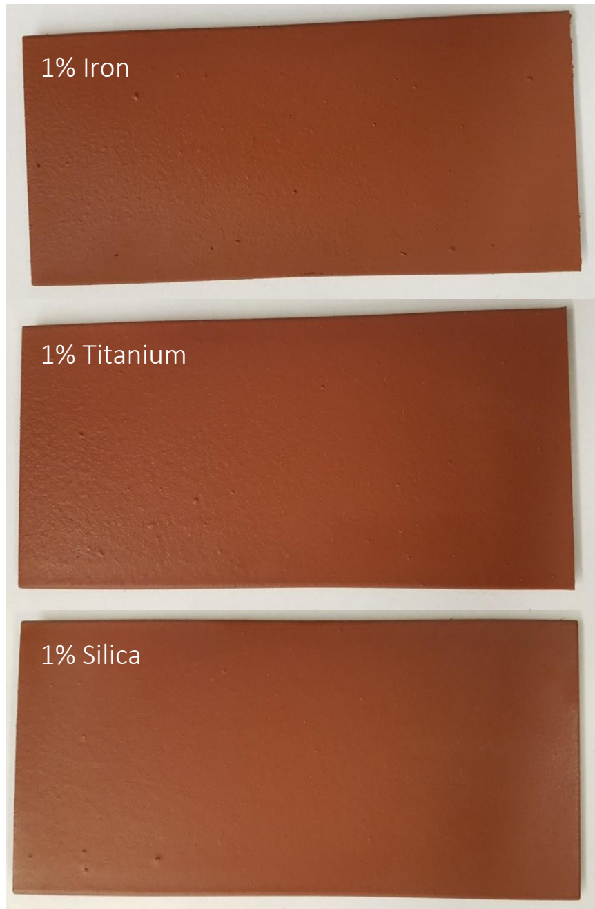
Figure 3-23 Cured Nano-Added specimens coated with spray gun.
