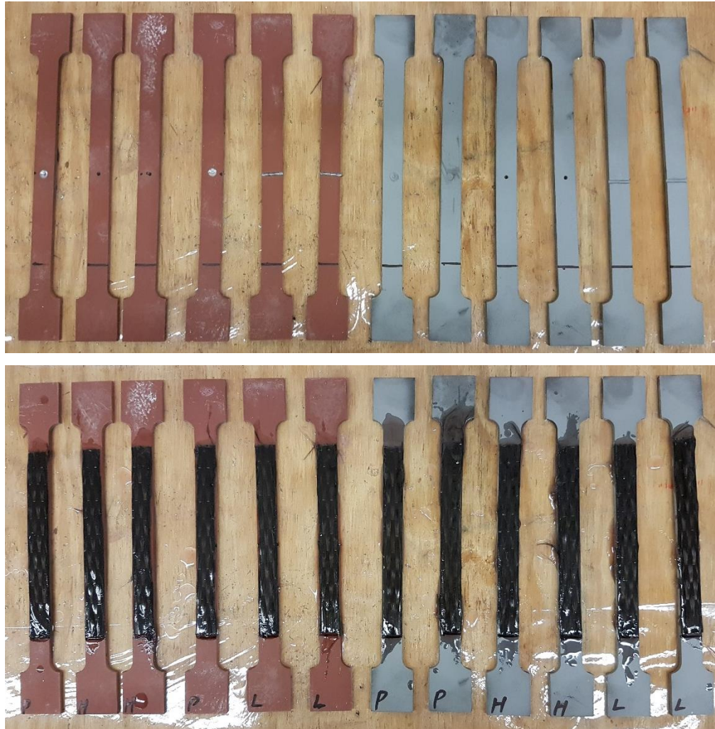
Figure 5-13 Types of damages (top) shown in the specimens, repaired specimens with CFRP.
