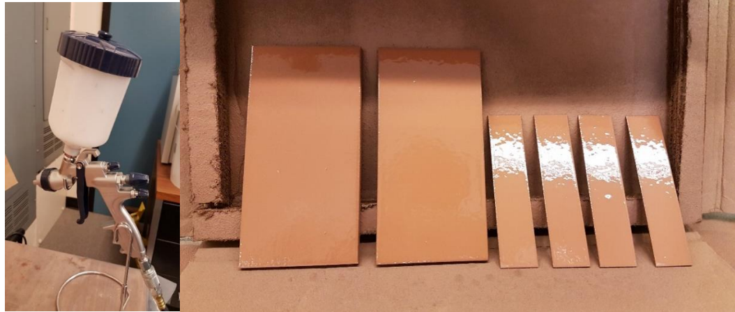
Figure 3-22 Fresh coated specimens using 1.4mm nozzle tip HVLP spray gun.
