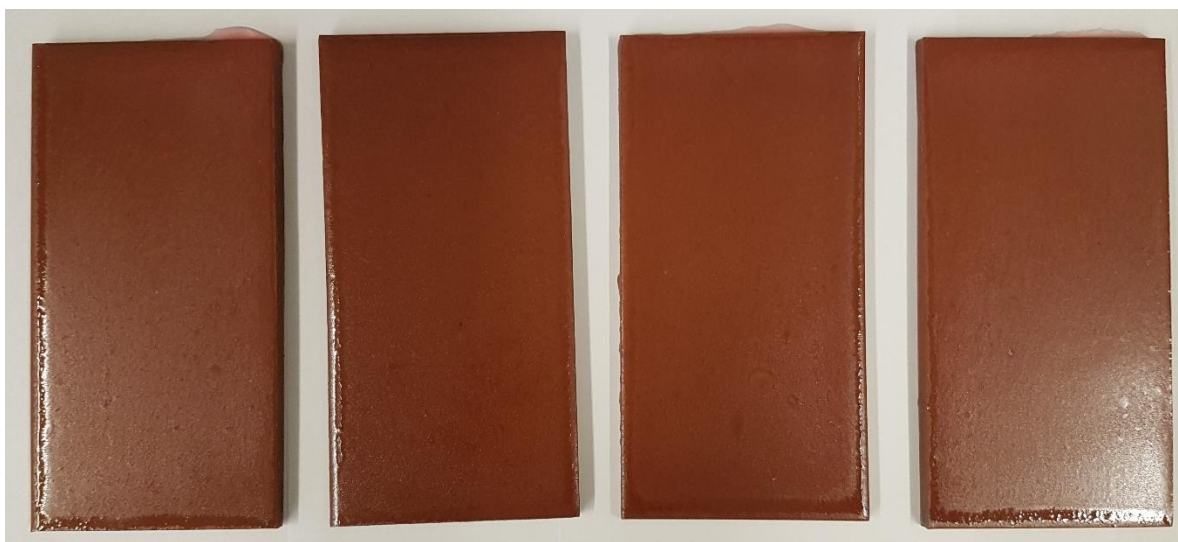
Figure 4-4 Resin Saturant applied and cured on coated samples.
