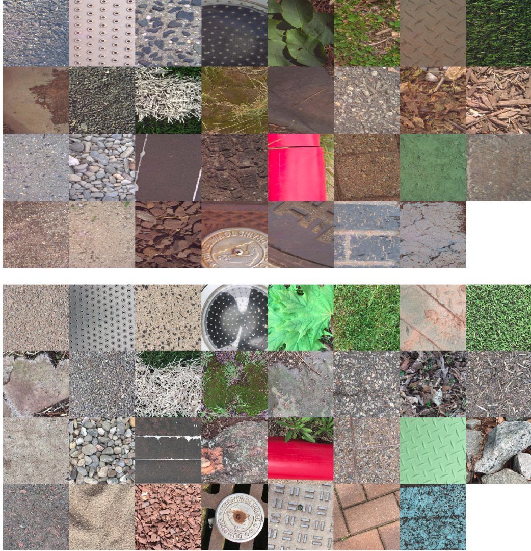
Figure 3.6: Comparison of images from the GTOS dataset (top) and GTOS-mobile (down) video frames. The training set is the ground terrain database (GTOS) with 31 classes of ground terrain images (over 30,000 images in the dataset). GTOS is collected with calibrated viewpoints. GTOS-mobile, consists of 81 videos of similar terrain classes captured with a handheld mobile phone and with arbitrary lighting/viewpoint. A total of 6066 frames are extracted from the videos with a temporal sampling of approximately 1/10th seconds. The figure shows individual frames of 31 ground terrain classes.
