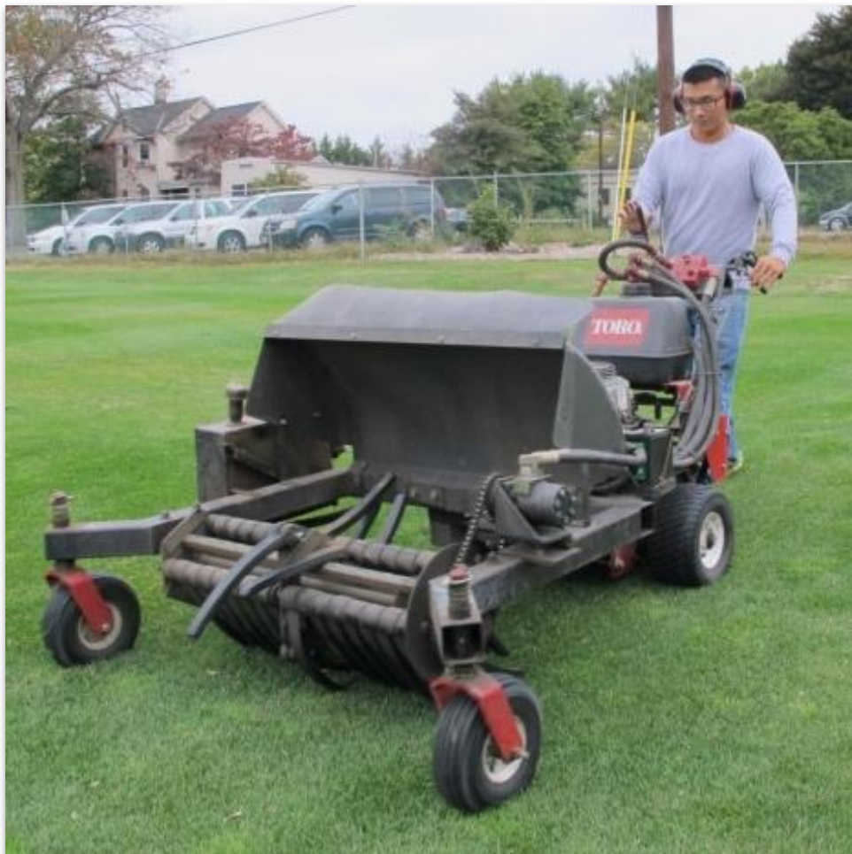
Figure 2.1 Abrasive wear applied with Rutgers Wear Simulator (RWS) developed by Bonos et al. (2012)
