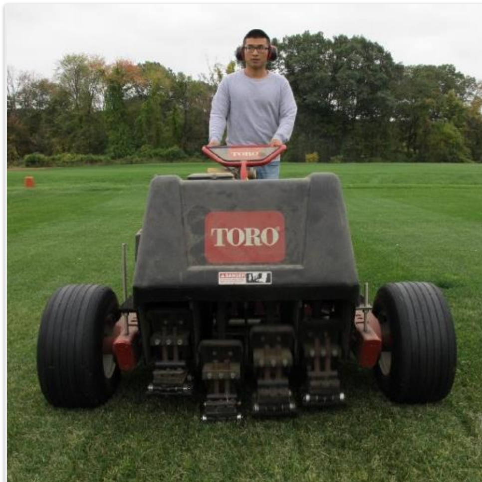
Figure 2.2 Cleated traffic applied with Cady Traffic Simulator (CTS) develop by Henderson et al. (2005)
